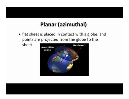
Now planar projection or Azimuthal projections, whereas I have said that we assume a flat sheet is located in contact with the globe, and points are projected from globe to the
