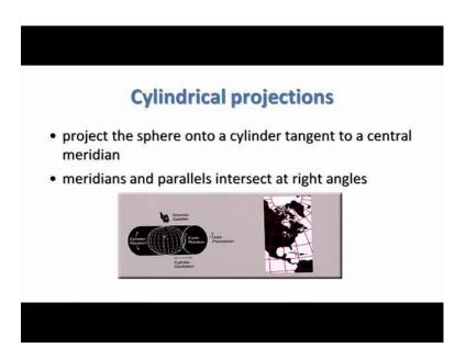
A cylindrical projection that sphere into a cylindrical tangent to a central meridian, and meridians and parallels intersect at right angles that you can see here. So, it depends on where exactly the cylinder has been assumed in this mathematical model.
