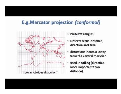
Mercator projection is also called conformal projections; this is how the distortions which are occurring to the Antarctica, but other countries are. In order to represent the true shape of Antarctica, it is better to have planer conformal or polar projections. We also call them polar projection, and when we assume when the sheet is kept at the say southern poles, and when the light is projected through the grid, then the true shape of Antarctica will come.
