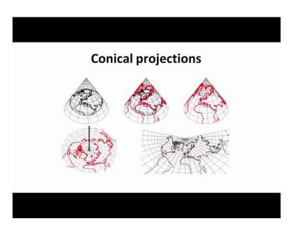
Now as I have said that it is need not to be that the cone of that paper has to be near the poles, you can make oblique projections, and depending on the again requirement, and therefore, things would be different. And this Albers equal area projection, conical projection will distorts scale, and distance except a long standard parallel.
