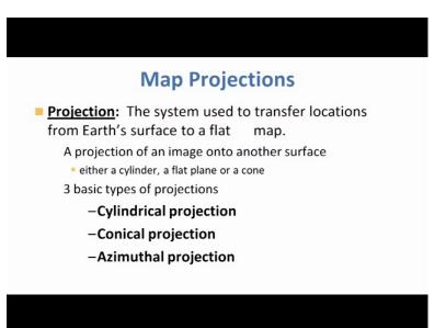
And projection of an image into another surface, either a cylinder a flat plane or cone. These are the basic types which have been we have already discussed, this one.
