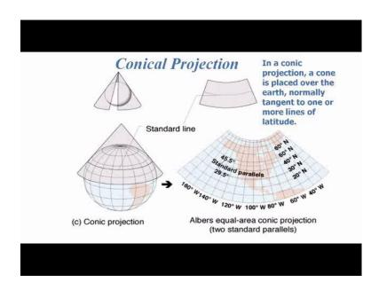
And then there are when we fix certain standard parallels, and with two parallel examples is given here, then this is called Albers equal area conical projection.
