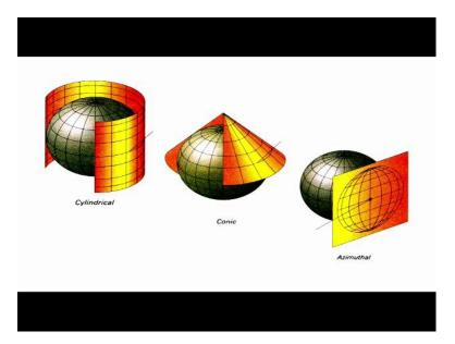
If I make that sheet as cone and then expose, then I would have in the center, the longitude would be radiating, from the poles, and then I will have circles for the latitude. Again in the Azimuthal projection, I am not going to say roll the sheet or make a cone or cylinder, instead if I keep just flat, then this is how it will be projected. So, these are the three basic types of map projection exists. Then there are variants, which we will see little later.
