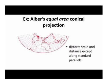
So, between roots two parallels which a user can give, as per the location of the country, between two parallels, these things can remain intact, but other things will get distorted.
