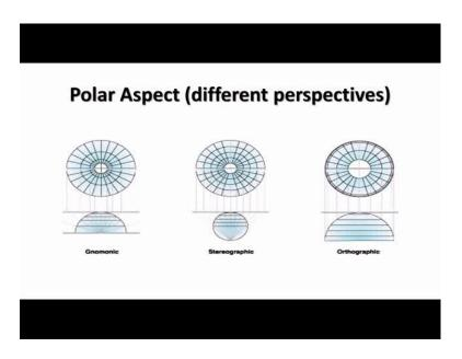
And then your stereo graphic projections are also used in geology, very common in structure geology for southern hemisphere, and also stereo graphic projections for northern hemisphere are used in mineralogy.
