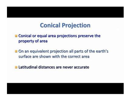
Now in conical projections also equal area projections preserve the property of area. On an equivalent projection all parts of earth surface are shown, with the correct area and latitudinal distance are never accurate. So, this is having problem with conical projections. Examples are here, that why these complications are there with conical projections.
