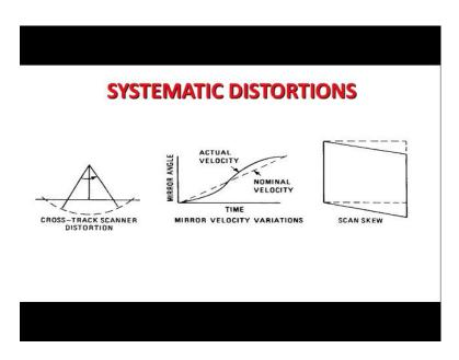
When sensors hit the mirrors, mirrors used to create velocity variations because these are all mechanical devices.
