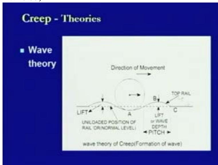
This is the normal rail level at this point. The dotted line is showing the normal level of the rail at which this wheel was placed. Now because of the loading condition there is this much deflection being caused in the rail section. So the rail section has bowed down like this at point A that is the point of application of the loading. Now when this has gone down in this form what is going to happen is a reverse curve gets formed like this.
