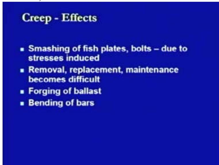
Because what will happen is that when the fish plates and the bolts will try to remain in their position because of no movement in the rail section but in the another rail section because there is a movement it will tries to create stresses and when this stresses become
