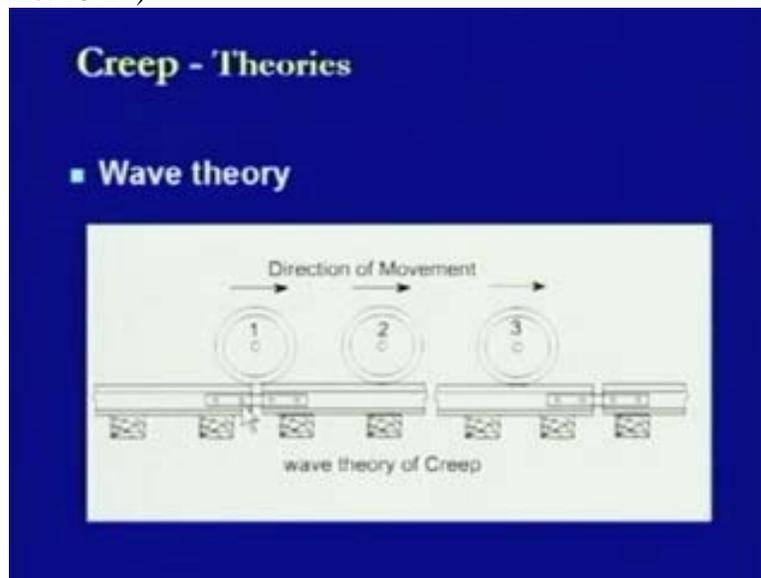
Now when there is number of wheels which are moving in this particular direction then what is going to be the effect of these wheels it is to be seen. Now what we see is that, now this is a condition which is happening because of a single wheel. Now this single wheel is being placed here and whatever load is being transferred this load is transferred at this position.
