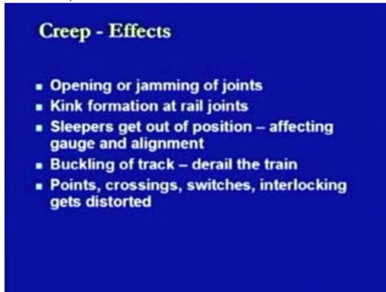
As the rail is moving it is trying to open out the joint at one end whereas it is trying to close the joint at the other end. Therefore, this is one of the effects which of the creep, that is, it will be opening the joint or it will be jamming the joint means it will just try to abort the 2 rail sections with each other and therefore the joints will not be there or there will be a problem associated with the movement of the rails with respect to the some other stresses.
