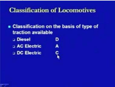
Further, on the basis of the type of the load which will be carried, we have A or L in case the light passenger, B or P in case standard passenger, capital C in case of heavy passengers, D or G for the standard goods, E for the heavy goods, M for the mixed conditions where the goods and passengers both are being transported and U, T or W
