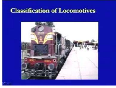
Similarly, there is a number being defined here is as 18527. 18527, the first three letters 185 they defines the series. It means it is 185 series locomotive and 27 means the production number. So, it in the 185 series it is 27 number of production of this type of locomotive of WDM2, that is how these numbers are defined and they are categorized.
