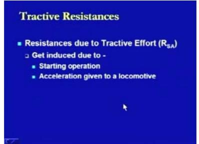
Here we will be looking at two conditions; one is because of the starting and other is because of the acceleration. In the case of the starting, the value is being defined for locomotives and for the vehicles, that is, the wagons differently and this is defined as point 15 w1 where w1 is the weight of the locomotive and in the case of the wagons or the vehicles it is defined as point 005 w2 where w2 is the weight of the vehicles.
