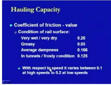
In the case of the condition of the rail surface, if it is very wet or very dry it is taken as point 25. It is greasy then it is taken as point 03. If it is average dampness condition then it is taken as point 166 and in the case of frosty or thermal conditions it is taken as point 125. Similarly, there is an effect of the speed and the case of the speed it varies between point 1 to point 2, that is from high speed to the lower speed conditions respectively.
