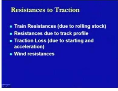
So, we come to the resistances to traction. In the case of resistances to traction as been shown in the previous slide or chart, what we have found out is that they are the train resistances which are due to the rolling stock, they are resistances due to track profile, the tractive losses which are caused due to the starting of the locomotive or the acceleration of the locomotive and the wind resistances.
