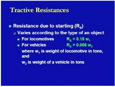
This is related to the starting, that is, the initial efforts which will be there. In the case of the acceleration, it is with respect to the change in speed ,that is, from v1 to v2 within a timeframe of time t. In that case this resistance is defined as point 028w into v 2 minus v1 divided by t.
