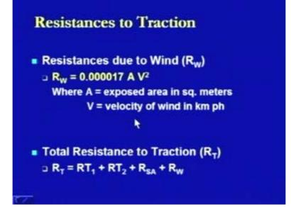
Therefore, the total resistance to traction will be defined as nothing but the combinations of all the resistances which we have seen so far ,that is, RT1, RT 2, RSA ,that is, starting an acceleration and RW, that is the wind effect.
