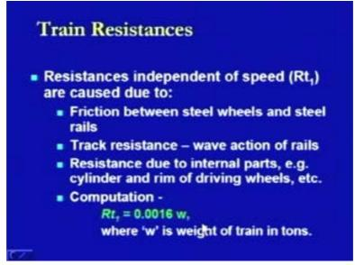
On all the basis of whatever types of the reasons are there which causes the this type of resistance the computed value of this resistance which is defined as a Rt 1 here is given as point 0016 w, where w is the weight of the train in tons. So, this is how all the efforts have been taken into consideration and finally this equation has been found out.
