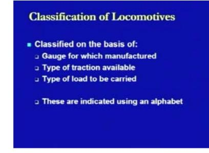
Now we come to the last thing in this case, that is the classification of the locomotives. The classification of the locomotives is done on the basis of gauges for which they are manufactured. The type of the traction available, the type of the load to be carried and based on all these conditions for which it is to be defined, they are indicated using an alphabet.
