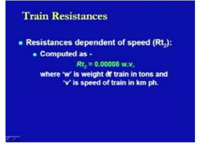
point 00008 w into v, where w is the weight of the train in tons and here what we found is from the previous formula now we are incorporating this vector v which is the speed of the train and that is how this is dependent on the speed.
