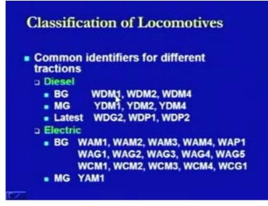
Just look at this locomotive, in this locomotive it is already written here as WDM 2. Now this WDM 2 means it is going to be used for a broad gauge because W, it is a diesel traction because of D, and this is M it means it can be used both for mixed conditions ,that is, for passengers as well as for the goods and 2 is the category means there has been the previous case also where WDM1 was also there.
