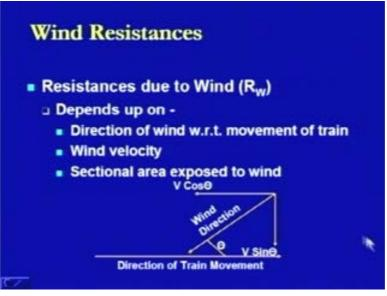
Now, there is another case of the wind resistance. In the case of the wind resistance it is going to be defined by certain factors like what is the wind velocity, what is the direction of the wind and what type of movement of the train is there with respect to that.
