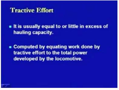
The tractive effort is usually taken as equal to or little in excess of the hauling capacity and this is computed by equating the work done by the tractive effort to the total power developed by the locomotive. So, this is the basis of the computation of the tractive effort for whatever the type of locomotive we are using, whether the steam locomotive or the diesel locomotive or the electric locomotive.
