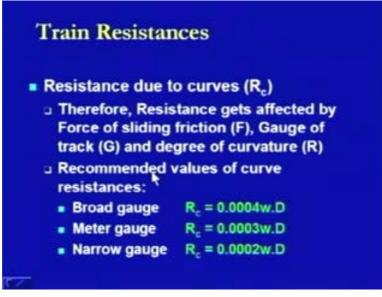
On the basis of the different competitions then the recommended values of the curve resistances have been given as such for the different gauges. For the board gauge, this value is 0.0004w into D, where D is the degree of the curve and w is the weight of the train. Similarly, in the case of meter gauge this factor changes from 4 to 3 and here in
