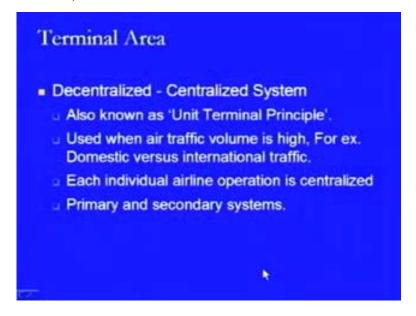
In the case of decentralized and centralized system it is also known as unit terminal principle. Here it is used where traffic, air traffic volume is quite high and it is one of the cases that we have the two types of traffics like domestic traffic and international traffic. So, in that type of a system, we can have a decentralized and the centralized system. So, we have the segregation of the two traffics by using this type of the system and each individual airline operation is centralized.
