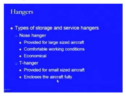
They are storage and service hangers like nose hangers, where they are provided for large sized aircrafts. Comfortable working conditions are there and they are economical, because only the nose of the aircraft moves into the hanger and rest of the aircraft remains outside. Further, there is a T shape hanger, where it is provided for a small sized aircraft and the enclosure is provided in such a way that the whole of the aircraft can come in.
