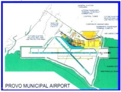
Here these are the air cargo commodity center where these can be controlled or these can be processed and then there is a permanent passenger terminal complex to come up in this location and then there is corporate hanger or there is another general aviation hangers being provided at this location. This is the apron area, this is the pury storage facility provided very near to the hangers, there are the hangers. So these are the things
