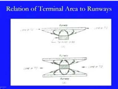
This is the case of a parallel runways system where this terminal building is being located in the center of these two runway strip, as we can see here. Again we can provide, we can use the runway hence both for landing or takeoff and there maybe landing or takeoff in this direction or landing or take off in this direction, again the multiple connectivity's have been shown as we have shown here.
