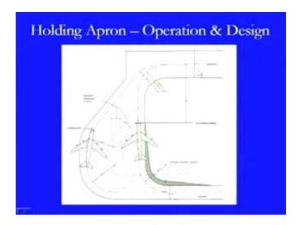
This is another diagram which tries to show the operation of different types of the holding aprons. We have seen the shapes of the holding aprons that trapezoid sort of holding aprons, or rectangular holding aprons which is being provided at the end of the taxiway and runway strip.
