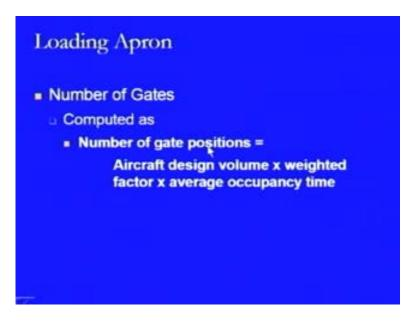
Now there are various models which can be used to find out the number of gate positions and some of them are being listed here; there is a Horonjeff model which is used in US, then there is a Piper modal in being used in Germany, there is Snow and Partners model being used in UK, then there is Loughborough model which is again used in UK and there is a Hart model which is being used in US.
