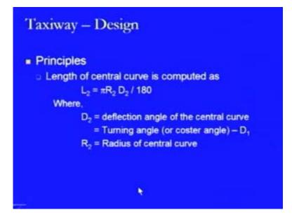
Now, the length of the central curve is computed by the formula pi into R 2 into D 2 divided by 180. So, these are all on the basis of the properties of the circular curve only. Now, here D 2 is the deflection angle of the central curve and this can be computed by taking the coster angle or the turning angle and subtracting D 1 from this value. R 2 is the radius of the central curve.
