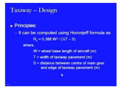
Then, this is, this R 2 value can also be computed by using the Horonjeff formula, which is 0.388 W square and this is divided by half of T minus S, where this W is the wheel base length of the aircraft in metres and T is the width of taxiway pavement in metres and S is the distance between the centre of main gear and edge of taxiway pavement, again in metres.
