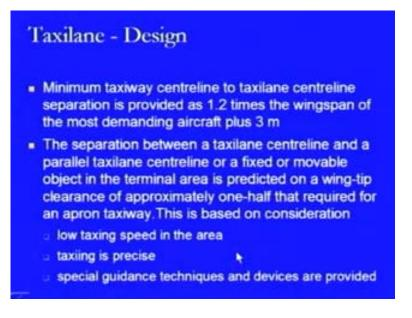
So, in this case, we have to design this taxilane. So, what we need to consider is that the minimum taxiway centreline to centreline to taxilane centreline separation is provided as 1.2 times the wing span of the most demanding aircraft plus 3 metres. So, that is how we can compute the value between the two centrelines. Then, the separation between the taxilane centreline and the parallel taxilane centreline or a
