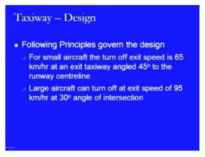
Now, we come to the design of the taxiway and there are certain principles which govern the design. In the case of small aircraft, the turnoff exit speed is taken as 65 kilometres per hour at an exit taxiway angle of 45 degrees to the runway centreline, whereas in the case of large aircrafts this turnoff speed at the exit time is taken as 95 kilometres per hour, where the angle of intersection is taken as 30 degrees. So, that is the rapid condition of the exit taxiway.
