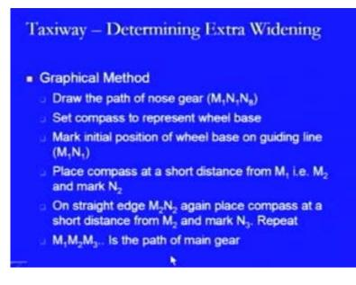
So, there is a graphical method of doing that and in that graphical method, first of all we draw the path of the nose gear, which say, being defined as M 1, N 1, N 8; N for nose gear, M for main gear. Then, what we do is that we set our compass to represent the wheel base which we have seen in the previous figure and once we have got this distance, then we mark the initial position of the wheel base on any guiding line and say that is M 1 N 1.
