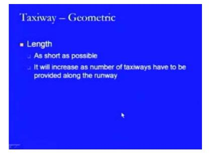
With this aspect in mind, we start with the geometric features that is the length. The length of the taxiway should be as short as possible. It will increase as the number of taxiways has to be provided along the runway, as we have seen in the previous case. There was a different connectivity, so it will increase the overall length of the taxiway.
