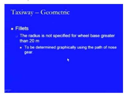
The radius is not specified for wheel base greater than 20 metres and it is to be determined graphically using the path of nose gear.
