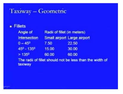
What we find is that for an angle of intersection between zero and 45 degrees, the radii of fillet in metres for a small airport is defined as 7.5 metres, for large airport it is taken as 22.5 metres, whereas if the angle of intersection varies between 45 degrees and 135 degrees, then the value for small airport is 15 metres, whereas for large airport that is 30 metres. Then, if the angle of intersection increases, it becomes more
