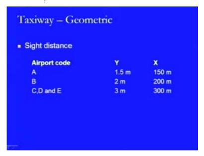
They have been defined with respect to the airport code that is the categorization of the airports and here for the airport code of A, the Y value that is the height above the pavement surface is 1.5 metres and in this case, the sight distance should be 150 metres, whereas in the case of airport code B, the height is 2 metres and the distance is 200 metres. For C, D and E category of the airports, the height is 3 metres, whereas the distance is 300 metres.
