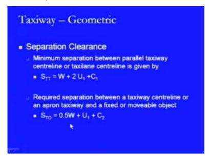
The minimum separation between the parallel taxiway centreline or the taxiway centreline is given by this equation that is the separation between the taxiways is equals to the W plus 2 U 1 plus C 1, whereas the required separation between a taxiway centreline or an apron taxiway and the fixed or movable object is given by, this is T and O that is object, then it is 0.5 W plus U 1 plus C 2.
