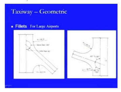
In the case of large airports, what we see is that again it is 135 metres or remains 60. If it is less than 45 degrees, then it becomes 22.5 metres. This is another diagram. As we have seen, for the smaller airports also, it is for 45 to 90 metres the radius is 30 metres as shown here and similarly for 90 to 135 degrees, the radius again remains 30 metres. So, this is the typical diagrams or typical connectivities, which can be provided.
