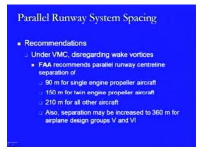
The recommendations here are that under VMC there are in respect to the wake vortices FAA recommends that there should be a centreline separation of 90 metres for single engine propeller aircraft, 150 metres for twin engine propeller aircraft, 210 metres for all other aircrafts and there should be a separation increased by 360 metres for airplane design group of V and VI category that is the bigger category.
