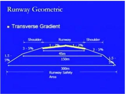
In this diagram, we look at the transverse gradients which have been specified. We have the runway strip being provided here along with some chamber at the centre, so that the water drains from to this side or to this side and the transverse slope being specified for this one is ranges between 1 and 2% and here, we are showing that this is having a width of 45 metres in the case of large airports, where the large aircrafts may be using the runway strip.
