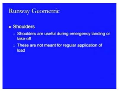
The shoulders are usually used for during the emergency landings or take-offs. That is the main specific function of the shoulders, but then they are not meant for the regular application of the load means during take-off or during landing, as on regular basis, they should not be used or otherwise they will deteriorate at a much faster rate, because they are not provided with the full strength pavement, as in the case of a runway strip.
