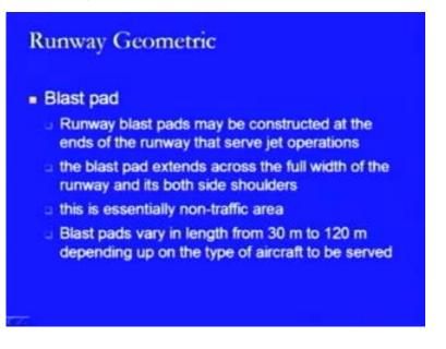
Then, the next aspect is a blast pad. In blast pad, the runway blast pad may be constructed at the ends of the runway that serve jet operations and the blast pad extends across the full width of the runway and its both side shoulders and this is essentially non-traffic area. We are not supposed to use this particular area for the movement. The blast pads vary in length and these varies from 30 metres to 120 metres depending on the type of the aircraft to be served.
