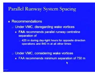
Here, in the case of VMC, the FAA recommendations are that the centreline separation should be 420 metres during day-light hours for opposite direction
