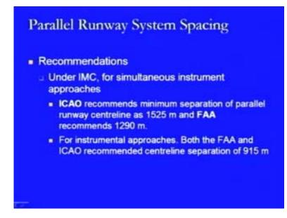
Then, in the case of IMC, for the simultaneous instrument approaches, the ICAO recommends the minimum separation of parallel runways centreline of 1525 metres, whereas the FAA recommends this distance as 1290 metres. In the case of instrumental approaches, both the FAA and ICAO recommend the centreline separation of 915 metres. So, these are certain recommendations as far as the provision of the different parallel runways are concerned.
