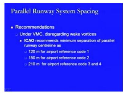
Further recommendations are that under VMC, we should disregard the wake vortices. Here, the ICAO recommendations are there which says that the minimum separation of parallel runway centreline should be as 120 metres for airport reference code 1, 150 metres for airport reference code 2 and 210 metres for airport reference code 3 and 4.
