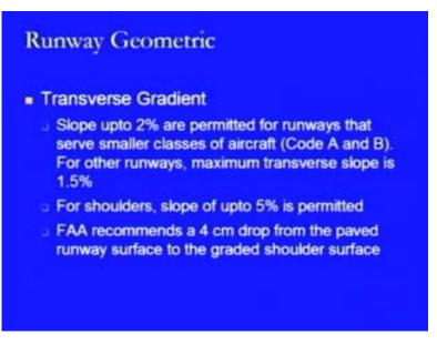
Then, a slope of up to 2% are permitted for the runways that serve smaller classes of aircrafts which are coded A or B, whereas for other runways the maximum transverse slope is fixed as 1.5%. In the case of shoulders, the slope of up to 5% is permitted. Federal Aviation Administration of US recommends a 4 centimetre drop from the paved runway surface to the graded shoulder surface. That is the specification by FAA.
