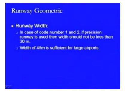
Then, further in the case of this code number 1 and 2, if precision runway is used, then the width should not be less than 30 meters. That is we are trying to define the runway in terms of the instrumentation condition, then the minimum width of the runway has to be 30 meters and in the case of large airports, the width of 45 meters is found to be sufficient.
