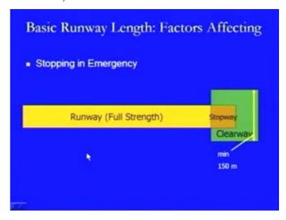
Now, this is how it looks like. This is the full strength runway strip and at the end of the runway strip a stop way is being provided and then, at the sides of this stop way and away from this one there is a clearway and this clearway again is having a minimum width of 150 meters. So, this stop way is also going to be a full strength condition.
