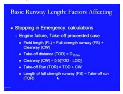
Now, here again these are the calculations. The engine failure take-off proceeded case field length is equal to full strength runway plus the clearway. Take-off distance will
