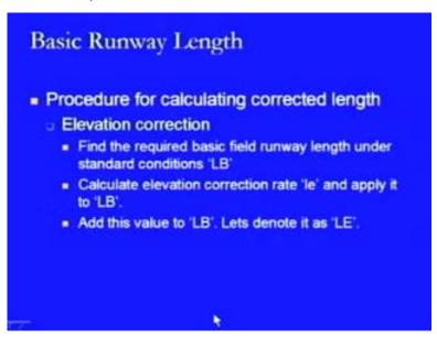
So, how we will be doing is this that first of all we have to go for the elevation correction. We find the required basic field runway length, which is required for mean sea level and under the standard conditions and say that is LB. Then, we calculate the elevation correction rate, small le and we apply it to LB and this will be the new value of the length of the runway strip and say this is LE. So, there is a, LE is nothing but LB plus small le.
