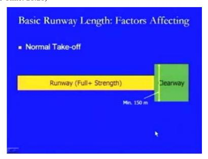
So, this is how it will look like in the plan, where this is runway strip and at the end of runway strip a clearway is being provided, where the minimum width of this clearway is 150 metres on this side and this runway strip is to be provided with full strength,
