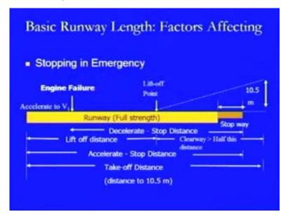
Now, this is a diagram which tries to show the same thing that the aircraft is starting from this location and then it starts accelerating. So, from zero value it is accelerating to a speed V 1 and at this point it is observed that there is a failure of engine.
