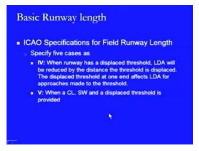
Then, the fourth case says that when the runway has a displaced threshold, then LDA will be reduced by the distance the threshold is displaced and the displaced threshold at one end will affect the LDA for approaches made to the threshold and the final case is that when the CL, SW and displaced threshold is provided, then we have to find out what is the length.
