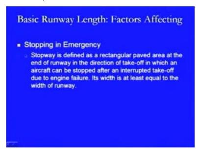
Now, this stop way is defined as a rectangular paved area at the end of the runway in the direction of take-off in which an aircraft can be stopped after an interrupted take-off due to engine failure and its width is atleast equal to the width of the runway strip or it may be more than that.
