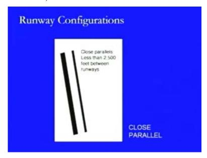
We look at the first case, where this is a closed parallel condition being defined on the basis of the distance between the centreline of one runway to the centreline of another runway and here it is being defined in terms of less than 2,500 feet between runways. If that is the case of the distance, then that is known as close parallels.
