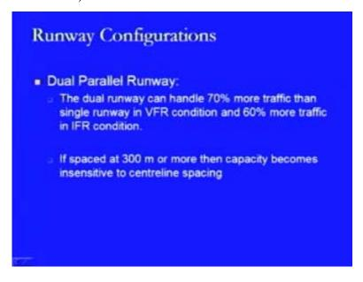
Capacity, as far as this is concerned, then it can handle 70% more traffic as compared to the single runway under VFR conditions and 60% more traffic than the single runway in case of IFR conditions and if spaced at 300 metres or more, then the capacity becomes insensitive to centreline spacing.
