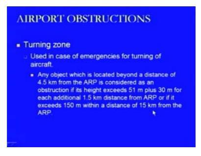
Then these are used in the case of emergencies for turning of aircraft and any object which is located beyond a distance of 4.5 kilometers from the ARP is considered as an obstruction if its height exceeds 51 meters plus 30 meters for each additional 1.5 kilometers from ARP. so if we are at a distance of 6 kilometers then it becomes 81 and so on and if it exceeds 150 meter with a distance of 15 kilometers from ARP. So this value remains the same as we have discussed in the previous case.
