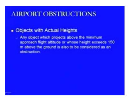
So, if we look at the flight altitude of the approaching aircraft to any of the airport and there is any object which is having a height more than 150 meter then that is also considered as obstruction.
