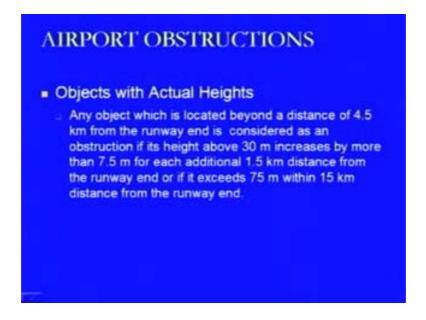
So within 37.5 meters height the development can take place but nothing can have a height of 37.5 meters or more than that. Similarly, when we reach value of 15000 meters or 15 kilometers from the runway and then it should not exceed the 75 meters value then if it is exceeding 75 meters than that an obstruction. Further, any object which projects above the minimum approach flight altitude or whose height exceeds 150 meter above the ground is also to be considered as an obstruction.
