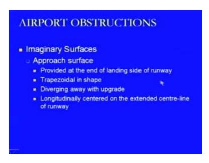
It is trapezoidal in shape, it diverges away with upgrade as we are going upwards away from the runway strip then it is diverging outwards. So that is how it is increasing in size. It is longitudinally centered on the extended center line of the runway. So it is with respect to the center line of the runway, it is symmetrical in location. This is another diagram which tries to show you the same of the thing.
