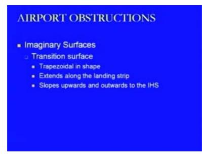
Then we come to another imaginary surface that is transition surface. This transition surface again is trapezoidal in shape and it extends along the landing strip and it slopes out upwards and outwards to the in inner side of the that is inner horizontal surface IHS, that is, what again we have seen that we go from the inner horizontal surface to the outer horizontal surface and it is extending in the outward direction and it is going up.
