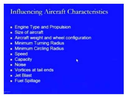
So we will take up one by one. The engine type and propulsion, this decides the size of the aircraft as we have discussed previously, the speed with which the aircraft can move obviously. The length of the runway because the more is the speed or more is the propulsion then the more longer runway strip is required for its movement so as to take off or so as to land and stop.
