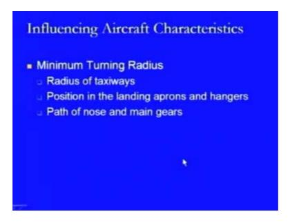
Now the next aircraft characteristic is the minimum turning radius and it has its effect on the radius of the taxiway. Taxiway is the connecting pavement which is provided between the runways and the aprons. The positions in the landing aprons and the hangers is also going to be governed by the turning radius that how they are going to be provided within the aprons or the hangers, the path of the nose and the main gears which will be traced on the pavement while it is taking a turn.
