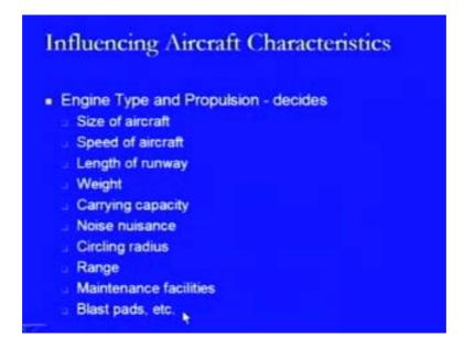
Then it also increases the weight of the aircraft with a bigger propulsion system or a heavier engine is being provided. It is also creating an effect to the carrying capacity of the aircraft because as we have seen it is creating an effect on the size of the aircraft. We are talking here in terms of the load taking capacity, the aircraft which is provided with the bigger engine or a better propulsion system can take higher load.
