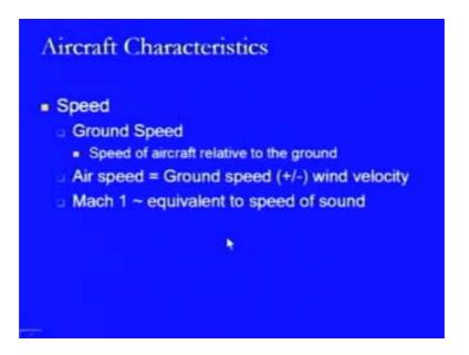
Generally they are being termed in terms of less than Mach value or more than Mach 1 value and on the basis of that we have the subsonic and supersonic aircrafts.
