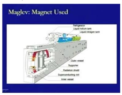
Here what we are trying, this is a refrigerator and this is a liquid helium tank and liquid nitrogen tank which is used to cool the superconductive magnet being shown here, with this is outer vessel, this is radiating shields, superconducting coil is being provided here. This is one super conducting coil and then this is inner vessel.
