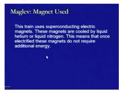
The amount of this attraction is so high that it can take higher, very, very high speed. This train uses superconducting electric magnets and these magnets are cooled by liquid helium or liquid nitrogen. This means that once electrified, these magnets do not require additional energy. This is another important thing. As soon as they get electrified, no additional energy is required to operate the system.
