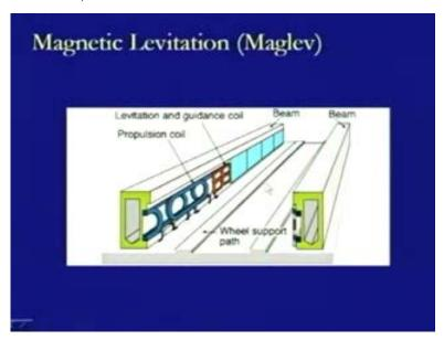
Then, another system which is used for the super high speed is the magnetic levitation in short known as Maglev. This is one of the costliest system, which uses the magnetic forces for propulsion as well as support and guidance and control and it is in general used as a design feature only. But now, China is implementing this one for looking at, to provide the connectivity from airports to the Olympic game village and travel will be through this magnetic levitation system.
