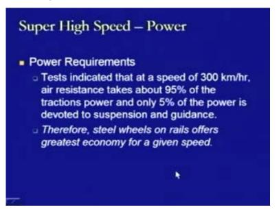
So, that is the amount of power which is being taken by the resistances and rest of the power which is available is very less for the guidance system. Therefore, steel wheels on rails offers greatest economy for a given speed.
