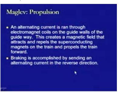
Similarly, we are talking about propulsion in this case. An alternating current is ran through electromagnet coils on the guide walls of the guide way and this creates a magnetic field that attracts and repels the superconducting magnets on the train and propels the train forward and the braking is accomplished by sending an alternating current in the reverse direction. That is how it is accelerated or deaccelerated.
