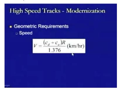
Then, in the case of the speed, the speed is computed by the formula as V is equals to C d plus C a multiplied by R divided by 1.376 and here the speed will come in kilometers per hour, where R is the radius of the curve and C a is the actual cant being provided or super elevation being provided and C d is the cant efficiency and this is the same formula which we have seen previously when we discussed about the geometric standards.
