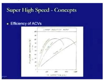
This is one of the graph which tries to define the efficiency of all these air cushioned vehicles, ACV's and here in this one, the correlation has been shown with respect to the speed on the x-axis and propulsive efficiency in percent on the y-axis. In the case of a linear induction motor, it is at 100% and goes constantly. That means whatever is the speed that value or propulsive efficiency remains constant, whereas in the case of turbo
