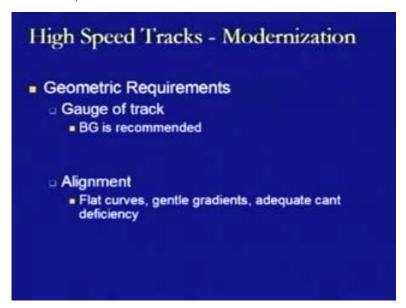
Now, we come to another requirement that is the geometric requirement. In the case of geometric requirement, the first thing is related to the gauge of the track, where the broad gauge is recommended. In the case of alignment, alignment should have flat curves, gentle gradients and adequate cant deficiency. Then only, the movement of the trains over the different type of alignments that is the horizontal alignment or the vertical alignment will remain in safe condition.
