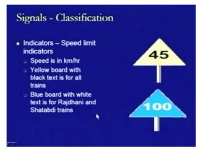
Then, we have some other indicators like speed limit indicators. So, if it is 45 means 45 kilometer per hour, if it is 100 means 100 kilometers per hour and yellow board is generally used for all the types of trains with black text, whereas if it is blue board with white text, then it for Rajdhani or Shatabdi trains. So, next time when you are moving, if you see this one, then you can understand this is the restriction for Rajdhani and Shatabdi and this is the restriction for rest of the trains.
