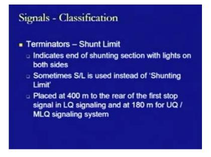
In this case this indicates the end of the shunting section with lights on both the sides and sometimes S of L is used instead of the shunting limit. So, that is how it indicates the termination of shunting area. Generally, it is placed at 400 meters to the rear of the first stop signal in lower quadrant signal system and at 180 meters for upper quadrant or M L Q signaling system, multiple signaling system.
