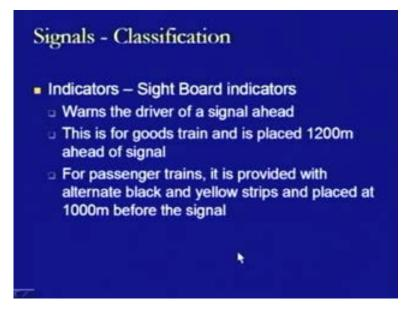
Then, we have the sight board indicators where which warns the driver of a signal ahead and this is for goods train and is placed 1200 meters ahead of the signal, generally and for passenger trains it is provided with alternate black and yellow strips and they are placed at 1000 meters before the signal.
