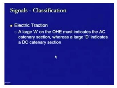
Then, further if there is a large A on OHE mast it indicates the AC, **whereas** if there is large D, .... it indicates a DC catenary section. So, this is how the electric traction indications are given to the drivers, when they are moving on electrified track. So, in this lecture as well as in the previous lecture, now we have seen regarding different type of signals which can be provided on any track.
