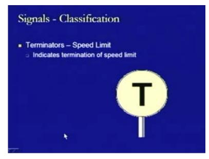
Then, we have another terminator which is speed limit terminator which is circular in section with T inscribed on that with a yellow background and black text. This is what is speed limit terminator. It indicates the termination of the speed limit.
