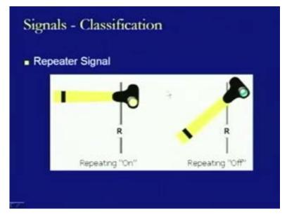
Then, this is another repeater signal which is provided in the form of movable arm and here it is yellow in colour and though this is semaphore type, but this is yellow with black band and here it is R being shown here and again the condition remains such that if it is ON position then it is horizontal stop condition, if it is inclined position means OFF position and proceed condition
