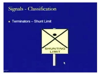
Then, this is a shunting limit terminator, as we have seen the B S L terminator, similarly in that sense this is cross means and this is written here.
