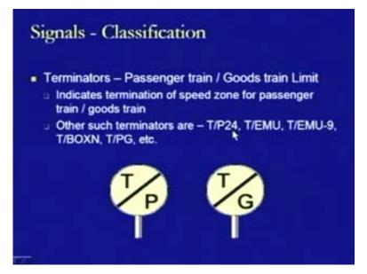
Then, similarly we have the terminators for say, for the passenger trains, for the goods train limits and they indicate the termination of the speed zone for passenger train or for the goods train. Other such terminators are also available like T oblique P24, T oblique EMU. That is EMU is generally used in the suburban or the urban areas like metros, etc. T oblique BOXN, this is BOXN for goods type of traffic, T oblique PG means passenger and goods and so on.
