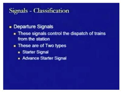
Now, we look at another category of signals that is departure signals. We have already seen the reception signals where two categories were there and that is how, the train is allowed to move into a station and occupy a platform. Now, we are talking about a condition when the train is standing on the platform and now it has to depart. So, at that location, at that condition whatever the signals are provided so as to dispatch the train
