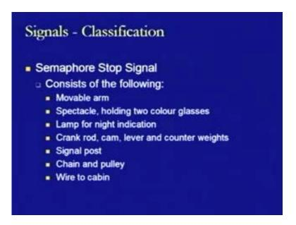
The components are the movable arm, spectacle holding 2 color glasses, lamp for night indication, crank rod, lever and counter weights working as a one complete assembly. Signal post, chains and pulleys so as to operate the movable arms and wire to the cabin from where it is operated. So these are the things which are provided in the case of a semaphore stop signal and that constitutes a signal.
