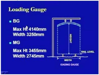
Then, there is a construction gauge. Construction is the gauge which is decided by adding necessary clearances to the loading gauge so that the vehicle can move safely without infringement.
