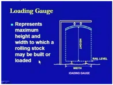
Now we can look at the specifications in the case of the broad gauge; the maximum height is 4140 mm where as the width is 3250 mm. In the case of the meter gauge, though we are of still continuing with the meter gauge that is why we are looking at this aspect, the height here is 3455 mm and the width is 2745 mm.
