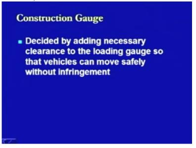
This is the condition which is to be provided in case of all the bridges or the tunnels or the pavements or the platforms which needs to be constructed or the shapes of all the platforms because there are certain clearances which are added to the loading gauge and then with those clearances this construction gauges is provided.
