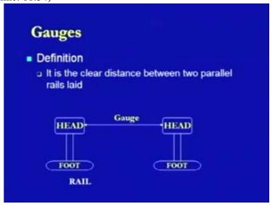
When we look at this classification, what we found is that they are different gauges which are available throughout the world. We have gauges like standard gauges. In the case of the standard gauges, the clear distance between the two rail sections is 1435 mm and these standard gauges are available throughout the world in on an average about 62 percent of the countries of the gauges which have been provided in the world, they are the standard gauges.
