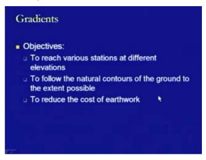
Now, why we are providing the gradients? Just look at some of the objectives of provisions of gradients. We are interested in reaching the different locations which are at different elevations. This is one of the primary objectives. Specifically in the case of hilly areas or in the case of the mountainous region or where the gradients are or where the cross slope of the ..... or where the topographical conditions are such that the two points at vast difference of elevation.
