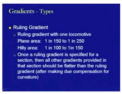
Then, in the ruling gradient, ruling gradient with one locomotive in the plane area is generally defined or restricted within the range of 1 in 150 to 1 in 250, whereas in the case of hilly area, it is 1 in 100 to 1 in 150. Now, once the ruling gradient is specified for
