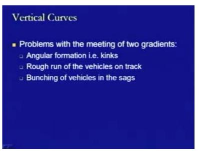
Another point, another problem which will be happening because of the gradients is bunching of vehicles in the sags. Sags are defined as the depressed portions of the gradients. What we can assume here is that if there is a falling line which is meeting the upward line, then the point at which these two lines are meeting that is there is a falling
