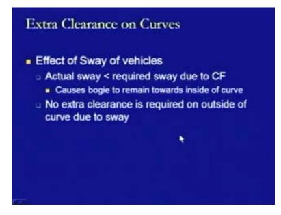
So, this effect of the sway of the vehicle what we found is that the actual sway is less than the required sway due to the centrifugal force. This is because what happens is it causes the bogie to remain towards the inside of the curve in this case and there is no extra clearance required on the outside of the curve due to the sway, because as this is the condition where we are talking about if the actual sway is less than the required sway due to centrifugal force.
