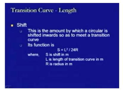
Now, we come to the length of the transition curve. The shift is already being defined and this shift is nothing but it is the amount by which a circular curve is shifted inwards, so as to meet a transition curve and its function is being given as S is equals to L square divided by 24R. This already we have seen, whereas S is shift in meters L is the length of the transition curve in meters and R is the radius in meter.
