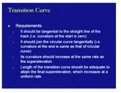
So, we have seen that there are three important things for which the transition curves have been provided - for the centrifugal force, for the smooth entry of the vehicles from the straight section to the circular section, for the uniform rate at which the curvature is being provided and as well as for the uniform rate at which the superelevation is to be provided. Based on these things there are certain requirements of transition curves. Now, we will look at those requirements now.
