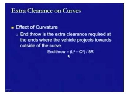
So, what we have seen here is that there is overthrow and which can be computed as C square divided by 8R and in the same condition of the effect of curvature, we can take up the another case that is the end throw and this end throw has already been defined in the diagram. It is the extra clearance which is required at the ends, where the vehicle projects towards outside of the curve and this is already been defined and this value is computed.
