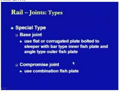
We will be looking at this combination fish plate when we take up the rail fastenings but just to mention here is that these combination fish plates are provided at those locations where the two rail sections which are being joined together they are of different sectional areas. So in those cases the normal conventional fish plates are not provided instead the combination fish plates are provided and at that location the joint which is provided is known as compromise joint.
