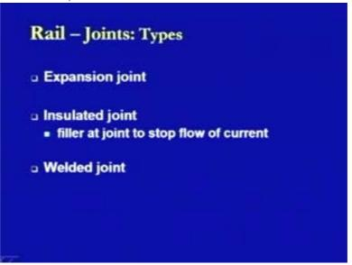
Then there is an expansion joint as we discussed it is provided so as to take care of the amount of expansion taking place in the rail sections because of thermal stresses.
