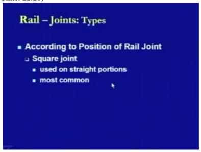
Then another one is on the basis of position of the rail joint. In this case the first type of a joint is the square joint. The square joints are mostly used on straight portions and this is one of the most common type of the joint which is provided on the railway tracks or the permanent way.
