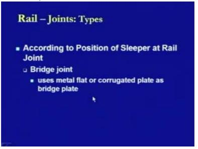
Then another type of a joint is known as bridge joint and in the case of a bridge joint we use a metal flat or corrugated plate which bridges the joint and that is why it is termed as bridge plate.
