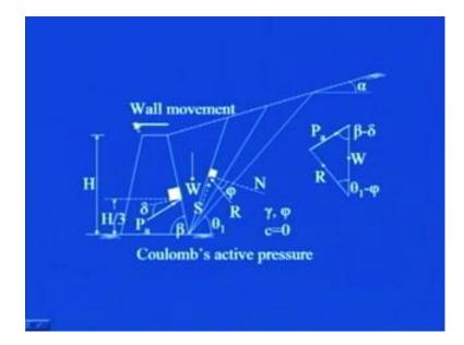
So, you see here this is a wall it is movement is in this direction, this is backfill, this is existing ground surface, this soil is backfill. So, you see the wall movement is away from the backfill, because of that the soil will form a triangular wedge right, it can fail along this wedge, it can fail along this wedge. This is not a fixed thing, but we talk in terms of any particular trial wedge and then we will try to generalize the process of analysis.
