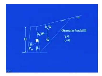
Now, let us see that how it comes into picture, we have already seen earlier that the weight of the wedge was the only vertical force, which was present when we were analyzing any trial wedge. So, in this case when the earthquake force is considered in that case and opposite vertical force of amount of magnitude K v into W is considered as shown in this figure. And then, an horizontal component of the weight W, which is K h into W is considered in this direction, that is in horizontal direction.
