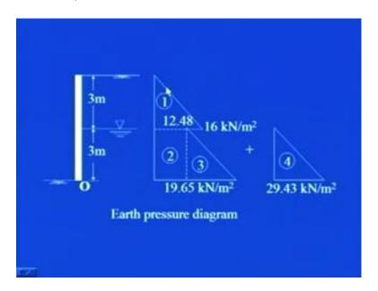
Now, you see here this due to this soil and this soil, since they are different the soil is also different and there is a presence of water table also. And we have found out that what is the pressure on top of this water table, what is the pressure in bottom of the this water table and then what is the pressure at the z is equal to 6. So, you see that from 0 to this z is equal to 3 your pressure was 16 kilo Newton per meter square, due to the soil which is present in the this top layer.
