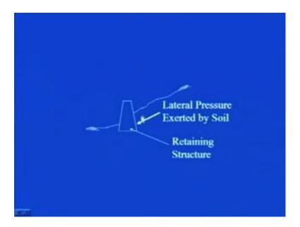
Now, first let us try to see I mean from common sense you can find out this soil is exerting lateral earth pressure on the wall. So, wall is always having a tendency to move away from the soil, in what case it will be moving towards the soil, now to explain this case let us try to have a look on this figure once again. This is what is the lateral earth pressure, which is exerted by soil because of this pressure this wall will have the tendency to move in this particular direction.
