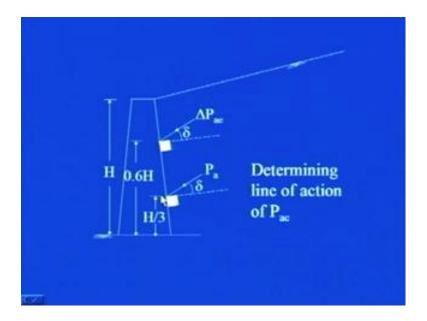
Then, what we do is we assume that this P a is acting at an angle of delta and at a height of H by 3 from the bottom of the wall.
