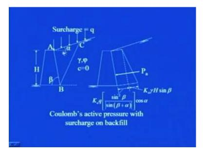
You see here, in earlier case the backfill was inclined and there was no surcharge present on that. In this case the Coulomb's theory is able to take into account plus the any surcharge, which is present on this inclined backfill, how it takes into account you can see here, that the backfill is cohesion less material that is c is equal to 0, it has unit weight gamma, you have angle of internal friction to be equal to phi.
