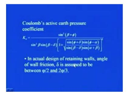
Now, you see the although the K a is coefficient of active earth pressure, but here it is how you can determine is little bit different from the Rankines analysis. Because, what happens is that Rankines takes care of the inclination of the back face of the wall plus angle of wall friction and all other this phi and beta aspect. So, you see this K a expression is given by this expression, it is not necessary to remember this long
