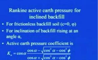
So, what will happen in that case, let us try to have a look on that, so your Rankine active earth pressure for inclined backfill, I assume that, usually in practice it is adopted that your backfill soil is frictionless. So, in case of frictionless soil, that is purely frictionless soil, your c becomes 0, it is just phi, which comes into picture, as for as shear strength properties of the soil is concerned. So, you see for frictionless backfill soil, your c become 0 only, phi remains there.
