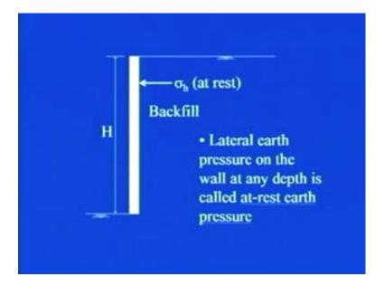
Now, you see that the lateral earth pressure on the wall at any depth, in this position of the wall is called at rest earth pressure. So, is this clear, in this one, the wall is not at all moving, now let us try to understand, that what happens if the wall moves away from the soil.
