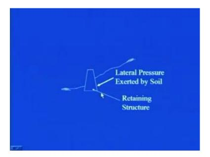
Now, let us see this, if I give there a retaining structure of this kind, then what is happening, the soil which was there about in this part. This is creating a lateral pressure, which will be resisted by this retaining structure and that is why it is called a retaining structure. So, you see that this retaining structure will function properly in the case, when this lateral earth pressure is estimated properly.
