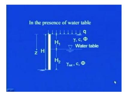
Now, I further complicate the situation that let us say that the water table is also present along with the surcharge. So, you see we are going step by step, first we saw that in K in the absence of any surcharge, only the wall was there and the backfill soil was there and then we saw that how we can determine the lateral earth pressure at rest condition. Then, we incorporate it, the surcharge on that, now it is the third step that, I incorporate the presence of water table.
