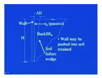
Now, the third one is when the wall is moving towards the soil, so you can see in this in earlier figure, the wall was moving away from the soil, in this case the wall is moving towards the soil. So, the wall may be pushed into the soil retain, there may be cases, I will explain you in the subsequent slides all those things. So, in this case the wall is moving towards the backfill soil and again I assumed that, this is the soil wedge failure; that is the triangular wedge is found.
