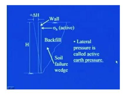
And the lateral pressure, in this condition is known as active earth pressure, now this one, we discussed, that when the soil is at rest, the second thing when the soil is moving, away from the soil.
