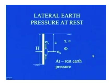
Now, after knowing all these three types of lateral earth pressure which can occur or which can act on a retaining structure, due to the presence of back fill. Let us try to analyze the case 1 by 1, that how exactly we can estimate the lateral earth pressure in these three different conditions. So, first let us try to have a look on the estimation of lateral earth pressure at rest condition, so you see, here is the wall, since it is at rest condition, it is not at all moving.
