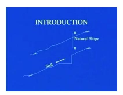
You can see that, there is a natural slope and if I cut it by a vertical plane x x as shown in the figure, it will result into this kind of situation and you can see that this soil above this part, will have the tendency to slide over. So, in case if you are planning to expand a road, then what will happen, this soil will slide over this road, which is an undesirable situation.
