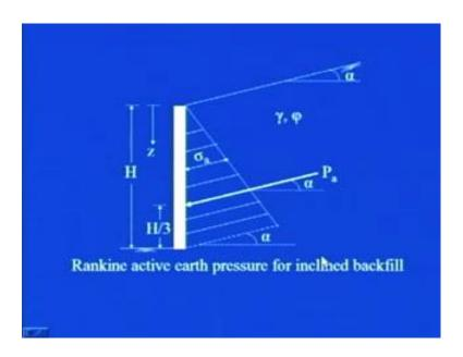
So, as you can see from this figure as I told you earlier, that this P a, that is total force, in case of an inclined backfill is acting at a distance of H by 3 from the base of the wall and it is parallel to the inclination of your backfill. So, you see at with depth, how it is changing and what is the value, that it will attain at this z is equal to H, along with this property of the soil as gamma and phi.
