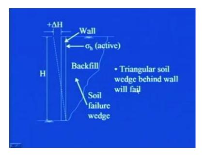
This condition is called active condition, you see a triangular soil wedge, behind the wall will fail.
