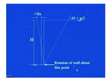
So, as we say that it is active pressure, you see wall is moving away from the backfill, Rankine assumed that the rotation of the wall, takes place along this point, which is at the bottom of the soil and the failure takes place along this failure plane, which makes an angle of 45 plus phi by 2 with the horizontal. So, you see the failure wedge which is getting formed is triangular in nature, that is this one and then delta x is the wall movement away from the soil.
