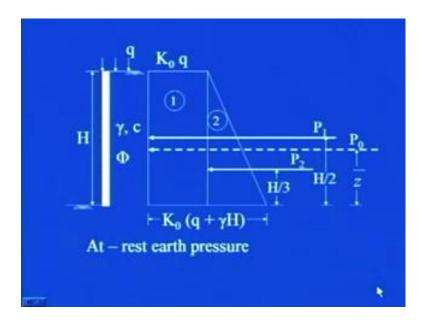
So, you see in K in the absence of any water table, just the surcharge has been added to the previous case as discussed earlier, what is going to be the difference, you see at the this particular depth, that is at z is equal to 0, your vertical stress is q. Now, if the vertical stress is q, wall is at rest position, what will be horizontal stress, it will be K naught into q. So, here at depth z is equal to 0, we plot it to be K naught into q.
