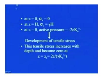
So, you see as I explained you, that at z is equal to 0, your sigma v is equal to 0 and so your sigma H is equal to 0, in that case at z is equal to H, your sigma v is gamma H at z is equal to 0, what is active pressure, you see here 0 minus this. So, that will be minus 2 c square root of K a, since it is with minus sign and you know that in soil is very good in
