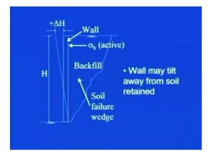
So, you can see here, that this is a kind of wall or retaining structure, then it is moving away from the soil by this delta H amount. Then, it will cause the soil to fail along this say soil failure, I mean it is not a very hard and fast that soil will fail along this failure
