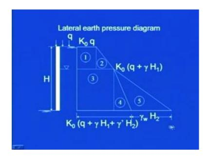
So, you can see, here I am showing you the earth pressure diagram in which surcharge is present and the water table is also present. So, you see first of all, I take a case above the water table, what is the vertical stress at z is equal to 0 is q only, so horizontal stress will be K naught into q. So, see I am showing it here, what will happen and z is equal to H 1, in this one, this is H 1.
