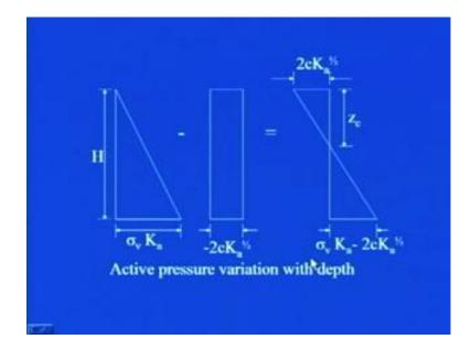
Now, how we can draw the lateral earth pressure diagram, because or it is always better to draw first earth pressure diagram, because after that your problems become very simple. That simply you have to take the area of that earth pressure diagram and then you will know the total force, per unit length of the wall and once the area is known. You can find out that, where are the different forces, which are acting and then you can find out the line of action of the resultant force.
