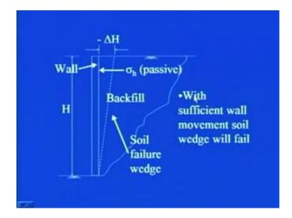
So, you see with sufficient wall movement the soil wedge will fail and in this case you can see here, this is the lateral pressure, which is acting upon the wall are retaining structure by the soil is called as passive earth pressure.
