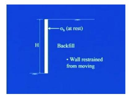
Now, as I told you that wall will have tendency to move upon the action of this lateral earth pressure, which will be exerted on the retaining structure by the soil. Now, the thing is that there can be three conditions either the wall is not at all moving or second thing wall can move away from the soil, that is away from the backfill or the wall can move towards the backfill. So, let us try to discuss 1 by 1, all these three conditions.
