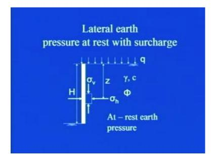
Now, we took a very simple case to make you understand, that what exactly do we mean by lateral earth pressure at rest. Many a times, it may happen that the backfill soil is subjected to some surcharge; it may be due to the existence of some structure some residential building or something like that. So, here I discuss a case, where lateral earth pressure with the presence of surcharge.
