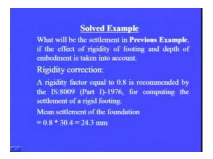
So, rigidity correction factor suggested by is IS 8009 part I 1976, it is 0.8, so mean value of settlement of the foundation will be equal to 0.8 into 30.4 that is the settlement we obtain from the from the De Beer and Martens approach using 1 q Es equal to 1.9 into qc upon sigma 0 dash. That, is comes out to be equal to 24.3 millimetre.
