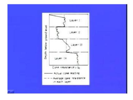
Now, here we divide this into number of layers having almost same value of Qc, so this is one such variation of Qc with depth in different layers. So, depending up on the variation, we can divide this in to number of layers and the average value is taken as the Qc for that particular layer.
