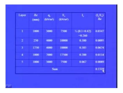
So, De beer and Martens has given this particular equation for determining the settlement of the foundation.
