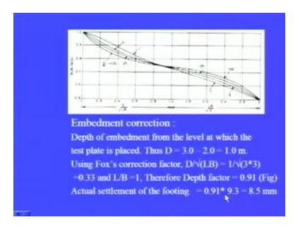
Now, then we apply an embedment correction in order to use this embedment correction, we use the chart which is given by fox and is recommended by IS 8009 part I 1976. So, from this chart, first of all we find out what is the depth of embedment and the depth of embedment is equal to 3 minus 2 that is equal to 1 meter. By using fox correction factor, first we find out D upon under root LB, so then D upon under root LB, it is equal to 1 divided by under root 3 into 3 that is equal to 0.33.
