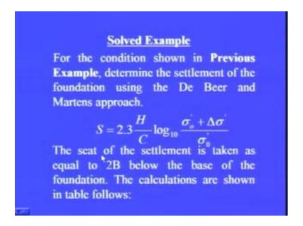
The seat of settlement is taken equal to 2 B below the base of foundation, the calculation are shown again in the tabular form in the next slide...
