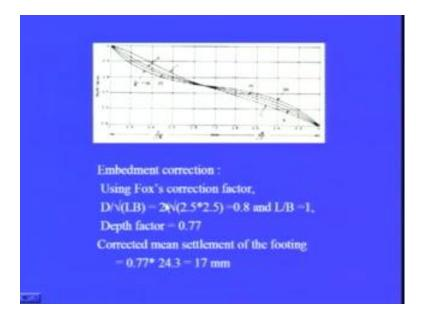
In order to apply the embedment correction factor, again we use the curve given in IS 8009 as suggested by fox and we find out first D upon root LB, so for this particular case it is 0.8 and L upon B equal to 1. The corresponding to this D root upon LB or 0.8 l upon B, using the appropriate curve, we find out the depth correction factor, we read from here
