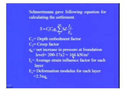
So, we divide this into number of layers and we use this Schmertmann equation to find out the settlement of the foundation, now in this case, even as said earlier C 1 is the depth embedment factor and C 2 is the creep factor, that we will determine q n is the net increase in pressure at the foundation level and that is equal to 200 minus 17 into 2, where 17 is the unit weight of soil and 2 is the depth of the foundation.
