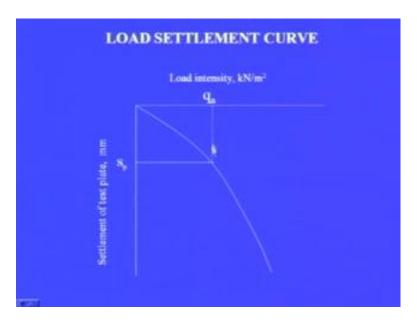
Now, a typical load settlement curve is shown here, here this is the load intensity kilo Newton per meter square and this is the settlement of the plate. So, corresponding to any load intensity, we find out the settlement of the plate and we get different points and we join them smoothly, we get the load settlement behaviour.
