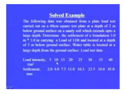
How to use this plate load test, for determination of the settlement of the footing resting on granular soil? The following data was obtained from a plate load test carried out on a 60 centimetre square test at a depth of 2 meter below ground surface on a sandy soil which extents up to a large depth. Determine the settlement of the foundation 3 meter by 3 meter carrying a load of 110 tonnes and located at depth of 3 meter below ground surface.
