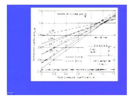
Now, for the circular footing as well as for the strip footing, so this coefficient mu can be obtained using this chart for the given value of the pore pressure coefficient a and depending up on the H the thickness of the clay layer and H by b ratio.
