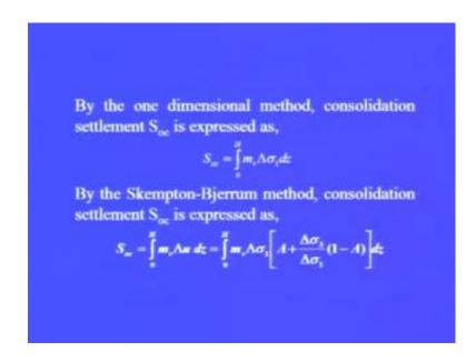
By the 1 dimensional method, consolidation settlement is expressed as, in terms of coefficient of volume change 0 to H mv delta sigma 3 dz, where d dz is the differential layer of consolidation. By Skempton-Bjerrum method consolidation settlement is expressed as this in in place of delta sigma. We substitute this as delta u and it will be equal to 0 to H mv delta sigma 1 A plus delta sigma 3 upon delta sigma 1 1 minus A into dz.
