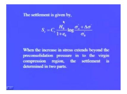
Then the settlement is given by Sc equal to Cr H 0 upon 1 plus e 0 log of sigma 0 bar dash plus delta sigma dash divided by sigma 0 dash. Now, when the increase in stress
