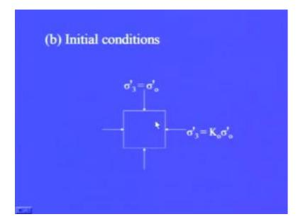
Now, initial conditions are sigma 3 dash equal to sigma 0 dash whereas, in the vertical direction. This can, we can determine as gamma dash into the depth under consideration of the point P, below the ground surface. And sigma 3 dash is equal to K not sigma 0 dash that is the lateral stress.
