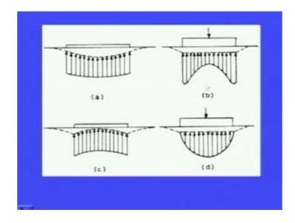
So, this is the case for the clays now, this is for the sand for the flexible and rigid footing.
