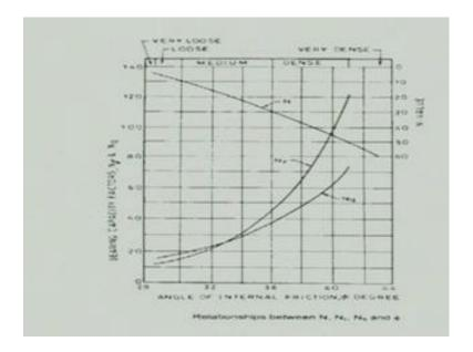
Now, this the graph for your reference projected again. In case of cohesive soils the bearing capacity does not vary with the size of the footing.
