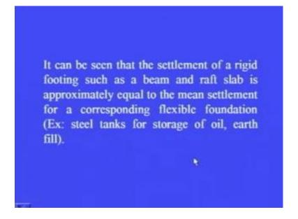
It can be seen that, the settlement of a rigid footing such as a beam and raft slab is approximately equal to the mean settlement for a corresponding flexible foundation. For example, steel tanks for storage of oil or earth fill are the examples of the flexible foundations.
