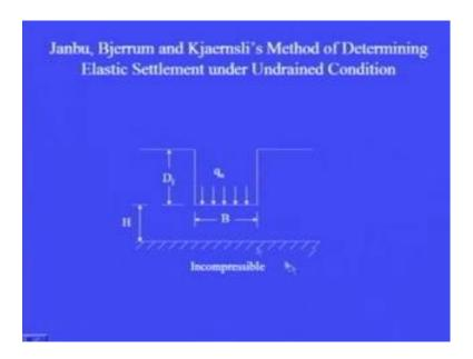
So, by this method we can determine Es there is another method suggested by Janbu et al for determining elastic settlement under undrained condition. Now, this is it can shows a foundation which is a which is placed at a depth of Df and the load applied to the soil is qn and width V is the width of the footing. And H is the depth of the soil layer below the level of foundation the this strata below this is incompressible.
