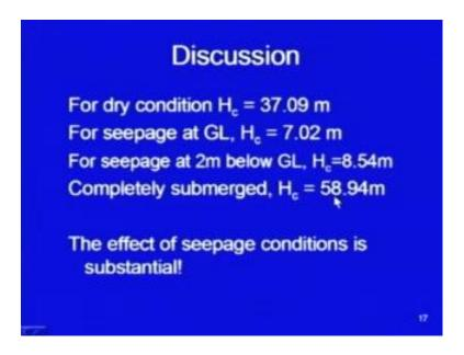
So, we have solved all the four cases and let us see it is interesting to see, what the results are? For the dry condition the maximum height for which the slope can remain stable was about 39 meter.
