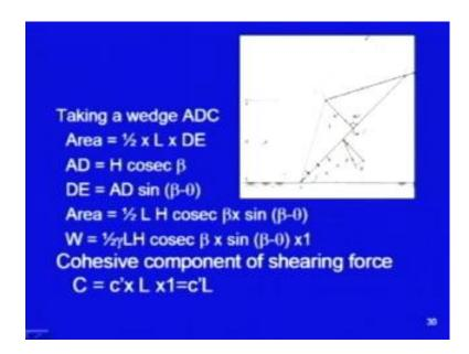
So, taking a wedge, this is the wedge we have taken and one can find out the area of this wedge and if you know the area you can find out the weight. So, weight area of this wedge will be equal to half into this base length into this perpendicular distance, so half into L into D E and this dimension A D can be obtained as now this angle is beta.
