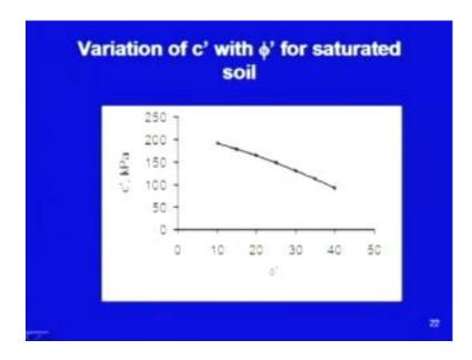
And here, the variation is plotted, on x axis it is phi dash, on y axis it is C dash and C dash you can see it is decreasing with increasing phi dash.
