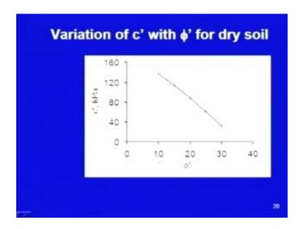
You can see it is decreasing, here I have shown the variation of C dash on y axis, we have plotted C dash on x axis we have plotted phi dash and you can see there is a variation of C dash with phi dash.
