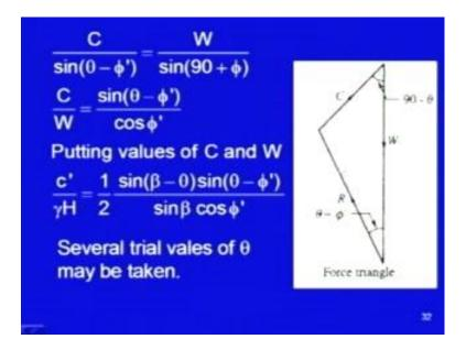
So, we now know the direction of this result resultant R and we know the direction of C, we know the direction of W. So, one can complete this force polygon, so this force polygon is completed.
