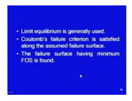
And again, limit equilibrium is generally considered as I told you limit equilibrium means we will be considering surfaces on those surfaces we will be finding out the shear strength. We will be comparing those shear strength with the applied shear stress and then we will know what is the factor of safety.
