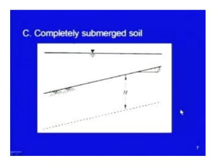
So, this was the case of partially submerged case, now I am taking third case here completely submerged soil. So, here the water table is not parallel to this, it is not seepage which is occurring here. In earlier cases, we were taking seepage to be taking place, whether it was through the entire mass or it was taking partially through the mass. Now, it is water table which is resting and the complete slope is now submerged, there will be difference now in the analysis.
