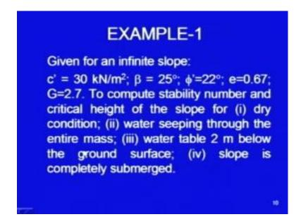
Let me now, solve some examples, it is given for an infinite slope, C dash is 30 kilo Newton per meter square. These are the shear strength parameters given for a particular problem, slope angle is 25 degree phi dash is 22 degree and e is word ratio is given as 0.67 and G value is given as 2.7.
