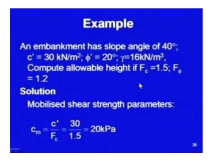
Lastly let me take an example, it is given there is an embankment it has slope angle of 40 degree, C dash is given as 30 kPa phi dash is 20 degree. The unit weight is 16 kilo
