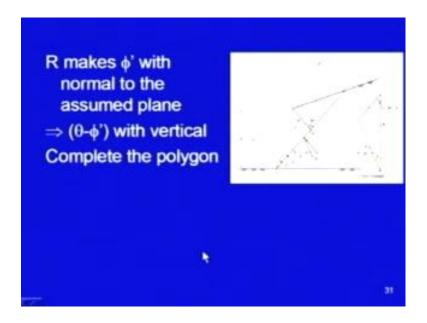
Now, we use a graphical method here, so in this case, this is the resultant R which has inclined at an angle phi dash with the normal. And so, you can find out the inclination of this resultant R, R is the resultant of the frictional component and the reaction.
