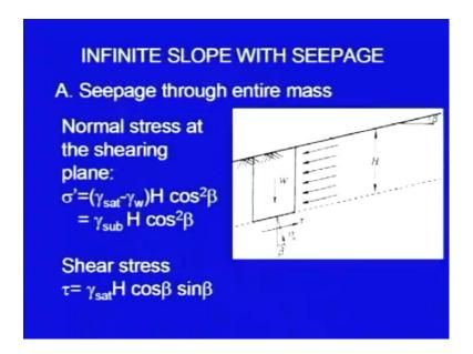
Now, let me take the another case of the infinite slope with seepage, here I be considering several sub cases. And first case I am taking seepage through entire mass, again this is an infinite slope, inclination is beta, depth is H and here is the plane of rupture on which we are considering the equilibrium and the seepage is taking place in this direction, we are considering this lies again it is weight will be acting in downward direction.
