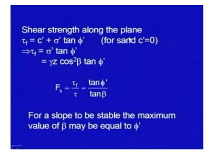
Let us get the shear strength along this plane, as I told you shear strength is the maximum strength which will be available. So, tau f will be equal to c dash plus sigma dash tan of phi dash and we are taking first example as the sand, so c dash is equal to 0 in case of the sand cohesion is 0. So, tau f will become sigma dash into tan of phi dash and
