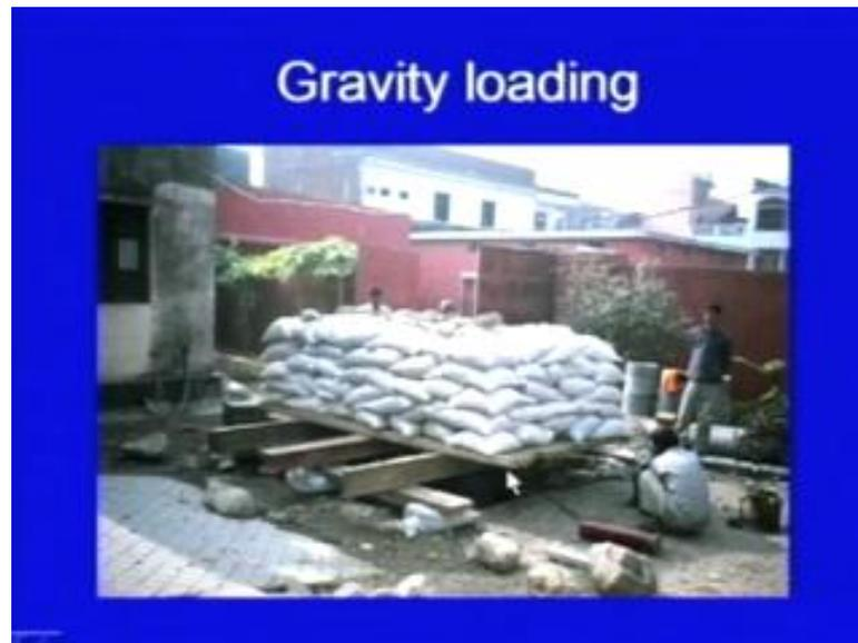
Here, it is a photograph which is showing the gravity loading, somewhere here there is a pit, it is going down; up to the proposed level of foundation and these are the girders. Cross girders are there; then planks are there, a platform has been made and on that platform, then sand bags are kept and using the weight of the sand bags, then we will be applying the load on the base on the plate.
