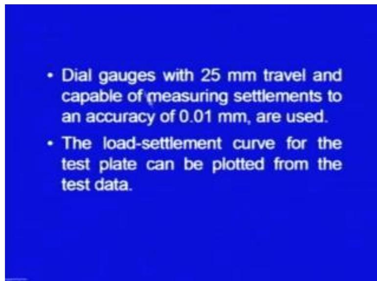
The dial gauges with 25 millimeter travel and capable of measuring settlements to an accuracy of point 0 1 mm is used. So, the important point is, we should measure the settlements to an accuracy of point 0 1 millimeter. This value can be more than 25 also and then from this test data the load settlement curve for the test plate can be plotted from this test data.
