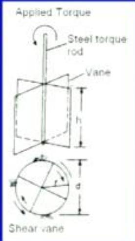
This vane shear, these are the vanes, it is it consists of four blades, first, second, third and fourth, these are the four blades and these blades are welded to a rod. And this vane is then pushed into the ground into the soil up to the required depth or at the bottom of the borehole. And then, at the top here, a torque is applied and there is an arrangement, which can measure the torque.
