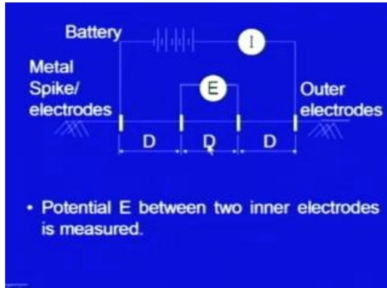
Here is the schematic diagram, this is the ground level and here are outer electrodes, this one, this one and then inner electrodes and in between these outer electrodes using a battery a current  $I$ ; is allowed to flow. By doing this, there will be a potential  $E$  between the inner electrodes, this is the potential  $A$  between this these two inner electrodes and this potential  $E$  is measured.
