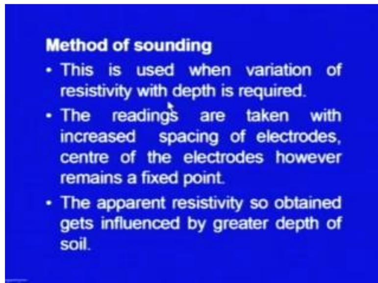
Now, this value is then, used to find out the soil types and there are two ways, first is method of sounding, this method is used when variation of resistivity with depth is required, we need the variation with the depth. In this case, the readings are taken with increased spacing of electrodes, centre of the electrodes; however, remains a fixed point. So, we keep the centre at a fixed point and we keep on taking we keep on increasing the spacing.
