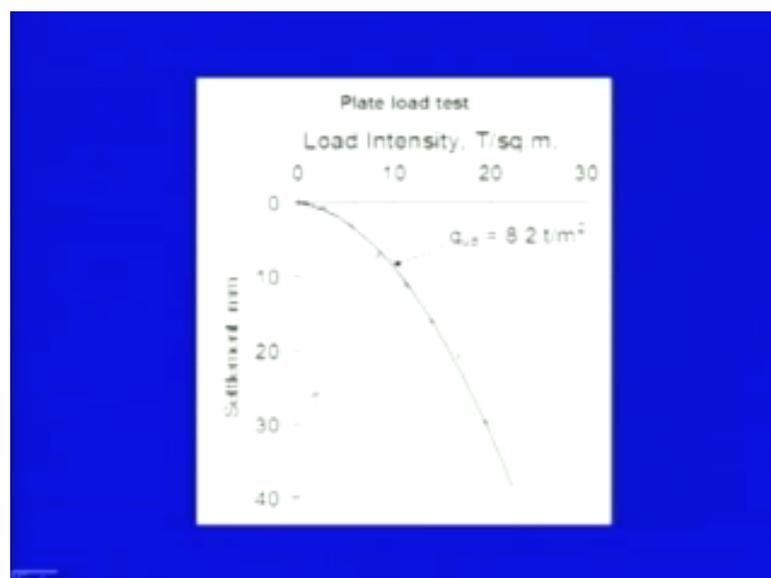
So, here I again, I have shown a graph, a plot and here I have shown how double tangent method can be used to find out the ultimate bearing capacity of the plate.
