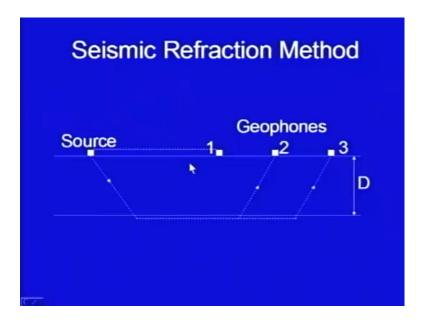
Let me explain it, using this particular figure, here is the source and this source is generating the waves, so what is happening is, there is one wave, which is directly going this way, it has certain velocity. Then, another wave, it goes into the ground and let us say here is a boundary of two different soils and then it gets refracted and goes to the geophone, these are geophones 1, 2, 3 and so on.
