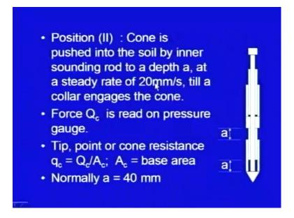
In the second step, the cone is pushed into the soil, this is the inner sounding rod, using this inner sounding rod, this cone is pushed into the soil, you can see now and this assembly was here, this entire assembly it was here. Let me show it again, here in this case, it was here and now it has been pushed using this rod by a distance a and there is a standard specified rate of 20 millimeter per second.
