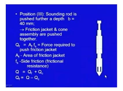
Now, come to the third step, let me explain what do you do in the third step first, this sounding rod is further pushed for a distance b which is again 40 millimeter and this time the friction jacket and cone assembly both they move. So, this will also be moving, this will also be moving, you can see this, so here the cone assembly as well as friction jacket both are moving.
