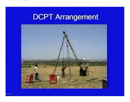
Here is a picture from the field, you can see here, this is the tripod, this one having these three legs and here is a arrangement pulley arrangement here. And here, it is being pulled by through this rope manually or here sometimes some arrangement is mechanical arrangement can also be made. So, this is the rope and here this is the hammer, this hammer is lifted for standard height, then it is allowed to fall.
