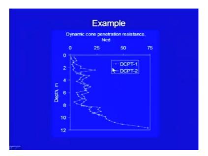
Here, I have taken an example, x axis is representing N c d and here it is depth, you can see there are two tests we have done. Now, in one of the test at two meter depth, there was sudden increase in N c d value, then it came down and then it was falling, this trend. The second test, which was done in the vicinity of the first test, was also having this kind of the trend, but it was not having large value at this particular place.
