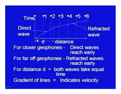
Here it is, I have shown the plot, here it is the distance, these are the geophones, 1, 2, 3, 4 5 and 6 and here I have plotted time. So, when you plot times for different distances, you will be getting two different straight lines, these two straight lines are meeting at this point, which is at a distance d away from the source. So, here it is the source and this is the point, where these two lines are meeting.
