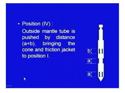
Come to now the last position last step, now this outside mantle tube is pushed by distance a plus b and doing that the friction jacket comes to the same position, which it was having in step 1, so this is pushed further and finally, it reaches this point.
