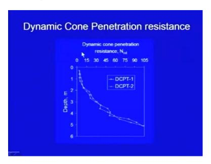
Here, it is an example I have taken from a field study, here on x axis, you can see there is dynamic cone penetration resistance N c d and this is for 30 centimeter successive penetration. So, 0, 15 and 30 we have taken up to 105 and here on y axis we have taken the depth and these were two tests, we conducted very close to each other.
