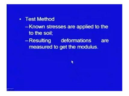
So, the philosophy of the test is that known stresses are applied to the soil, in fact to the walls of the borehole, resulting deformations are measured and then we get the modulus.
