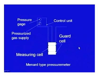
I am not going in detail for this test, just philosophy is being discussed here, this is the schematic diagram of this test, here it is the ground level and here it is a borehole. And in this borehole, here this is the measuring cell; these are the guard cells at the top and bottom. And then, pressure is applied, because of this pressure, there will be some deformations in the wall.
