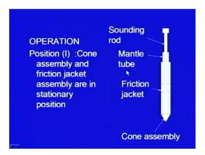
This is the operation, the operation of this test has been explained in four steps, this is the first step, which I am calling as position number 1, this is the cone assembly and here it
