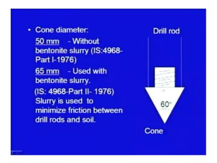
Here, I have shown the cone which is attached to drill rod, this is the cone and it is attached to this drill rod, this is the drill rod, apex angle of the cone is 60 degree and the diameter of this cone standard diameter is 50 millimeter. When, it is used without bentonite slurry as per this IS code, IS 4968 part I, 1976 and sometimes another diameter it is also recommended by the code, the diameter is 65 millimeter it is used, when the bentonite slurry is used.
