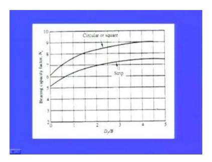
We can use this particular plot between bearing capacity factor Nc and Df by B and D from using this, particular graph, we can obtain for different values of D by f B D by Df by B ratio.
