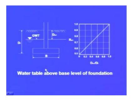
Now, this Rw 1 and Rw 2 can be obtained using this chart; you can see from here this is the depth of foundation. This is width of foundation, this is the position of the ground water table, which is at a depth Dw 1 below the ground surface and using this chart we can find this, Rw 1 depending upon Dw 1 by Df ratio.
