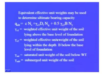
Another method, for considering water table is by making use of equivalent unit weight effective, unit weight gamma e 1 and gamma e 2. And these equivalent effective unit
