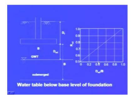
Similar to this, if suppose water table is below the base level of the foundation. And it is at Dw 2 below the base level. Then and it is within the width, within the depth equivalent to width of the foundation, then we can use this particular chart to find out Rw 2. So, here, Rw 2 can be read or it can be calculated by the equation which we discussed in the last lecture.
