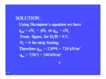
Now, using this chart and the equation given by Skempton we have find out this q ultimate equal to cNc plus gamma Df where this Nc is obtained by the previous chart and as it is on the surface. So, this Df equal to 0 we will end up with q net ultimate, that is equal to cNc. Now, from this figure for Df by B equal to 0.5 Nc comes out to be 6 for square footing strip footing therefore, q ultimate equal to 120 into 6 that is 712
