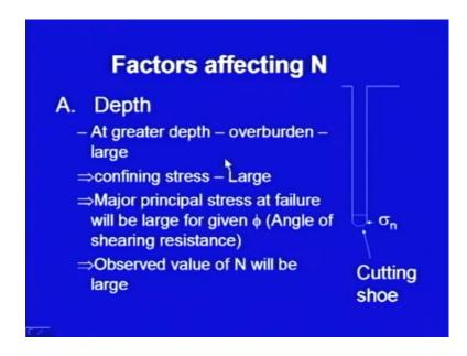
Let me discuss some factors which affect and because, we are going to use, we are going to correct this n for those factors, the first factor is the depth at which we have conducted the test. Now, here I have shown a bore hole and here there is a cutting shoe, cutting shoe is cutting this soil the soil is failing here and let us say there is some depth here, this is the depth at which the test is being conducted.
