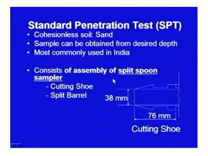
Let me start with the first one Standard Penetration Test SPT, this test is a basically or it is applicable mainly for the cohesionless soils, for example sands and as I discussed it is conducted in the bore hole. The samples can be obtained from the desired depth and probably this is the most commonly used test for sands in India, the most important part of this test is assembly of split spoon sampler, this is the assembly.
