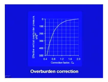
Here is that chart, you can get this chart in any of the standard book, on x axis the correction factor is there, it is varying here from 0.4 to 2.0, on y axis it is the effective vertical overburden pressure in kPa. And you can note down that when the pressure is between 0 to 100 kPa this is the standard value and at 100 this value correction is exactly 1.0, so no correction is applied for effective overburden pressure equal to 100 kPa.
