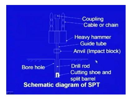
This is the schematic diagram of the standard penetration test, here this is the ground level and there is a bore hole, the bore hole has been advanced to certain depth, normally we do it at certain intervals. For example we start with let us say 0.75 meter depth below the ground, next test we take at 1.5 meter, then at the interval of 0.75 meter or as the depth increases we can increase the interval.
