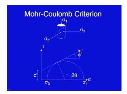
Let me go little bit more in detail about the Mohr-Coulomb criterion, I have shown here a soil specimen sigma 3 is all round pressure and considering it now in 2 d only, so sigma 3 is acting in this direction, sigma 1 is acting on this direction. And let me take a plane which is inclined at theta degree with the horizontal, theta it is making an angle theta with the plane on which sigma 1 is acting.
