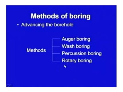
There are several methods of advancing the bore holes, first method is auger boring, wash boring, then percussion boring and rotary boring.
