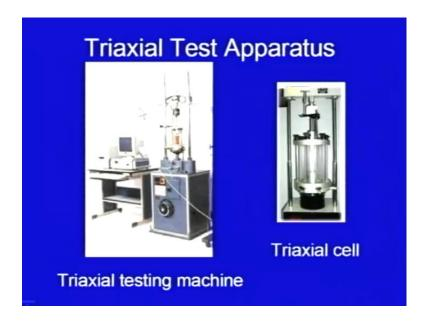
Here are some pictures of the triaxial test apparatus, this is the triaxial testing machine it is having a loading frame and most important part is here it is shown here triaxial cell, in this cell the specimen will be placed here and using water all round pressure sigma 3 will be applied and then, the load will be applied. So, corresponding to different sigma 3 you can go on increasing the deviatoric stress from the top up and you can continue up to the failure occurs.
