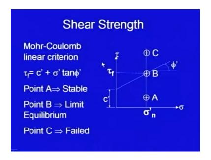
Let us talk about this failure envelope, the most widely used expression for this failure envelope is Mohr-Coulomb failure criterion, this is a linear equation. Mohr-Coulomb equation uses two parameters, C and phi or C dash and phi dash, wherever it is applicable. The equation is given as the failure, the equation of the failure envelope is given as tau f, here it is y axis has shear stress, tau f is equal to c dash plus sigma dash tan phi.
