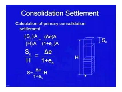
Here, I have shown the soil mass of depth H and some let us say a building is constructed over here and because of that load there is settlement, one can get these expressions, this
