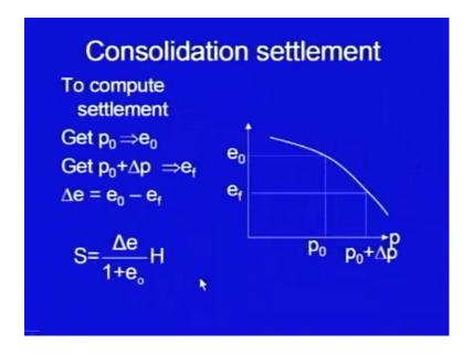
How to use this expression in the field to compute the settlement, what we do is we get the effective pressure at that particular depth, where we want to calculate the settlement. And corresponding value of e 0 we read from e versus log p curve, this is again the same curve y axis is e and x axis is on log scale is pressure, so corresponding to p 0 you can find out what is the void ratio e 0, this is the initial void ratio.
