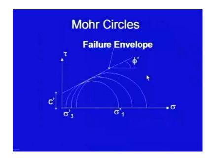
The results of the triaxial test will be available in terms of the confining pressure and corresponding deviatoric stress from which you will be able to calculate the major principles stress. Now, if you conduct test on different confining pressure values and plot them on Mohr circles, you know Mohr circles it is a sigma axis and here it is tau axis, on sigma axis you can put sigma 3 here and sigma 1 here and then, take this as the diameter and draw the circle.
