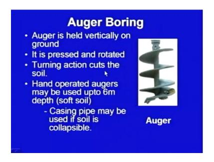
Let me in brief discuss all these methods, in first one the auger boring this is a picture of the auger, this auger is held vertically on the ground and it is pressed and rotated, here it is the cutting edge the turning action cuts the soil and that soil is excavated out. So, these augers hand operated augers can be used for shallow depth, for greater depths you have to use the machines, so this is the first one.
