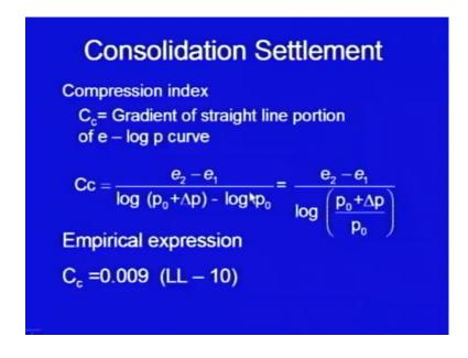
Now, let us go to the parameters which we can compute from this test, one of them is compression index we shall be using compression index to calculate the settlements and it is defined as the gradient of the straight line portion. You take the straight line portion at the higher pressure values and then, find out its gradient from the previous curve which I just discussed.
