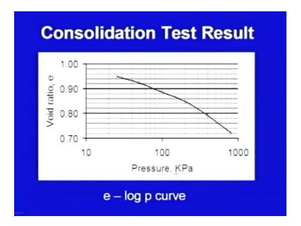
Here on the x axis it is the pressure, remember it is effective pressure, means total minus in the field when you use it you have to use the effective stress here. So, it is the effective pressure and on y axis we have the void ratio and this is the way the variation of e has occurring with pressure p, so this is the output, one of the outputs of this particular test.
