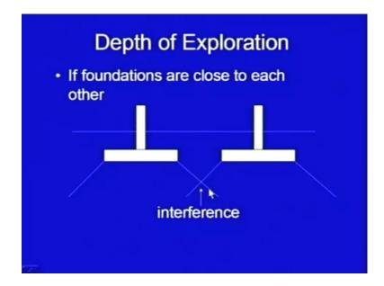
Here we have shown these two foundations, if they are closed to each other this is the stress of deviation, the stress is being dispersed in this way, so somewhere here the interference is start, so in this case you should have much more data available up to much more depth.
