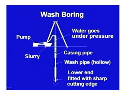
Wash boring technique is used this is a tripod having some pulley arrangement, here is a pump using pump, water is forced through this casing pipe and at the lower end, the end is fitted with sharp cutting edge, so water is there and cutting edge is there.
