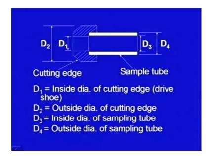
Here I have shown a sampler this is a cutting edge here, this is the sampling tube, D 1 is the inside diameter of the cutting edge, so sample will enter, the soil sample will enter from here towards this sample tube. D 2 this is the outside dia of the cutting edge, so this particular cutting edge this enters the soil first and soil specimen, the soil sample will be collected at this place. D 3 is the inside dia of the sampling tube and D 4 is the outside dia of the sampling tube.
