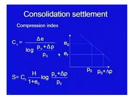
If you are using the compression index as per the definition of the compression index C c is delta e upon log of p 0 plus delta p upon p 0, it is the gradient of the straight line portion. We combining this equation and the previous equation of the settlement I can get this expression for the settlement S is equal to compression index multiplied by thickness of the, layer for which you are calculating settlement divided by 1 plus e naught it has the initial void ratio this one.
