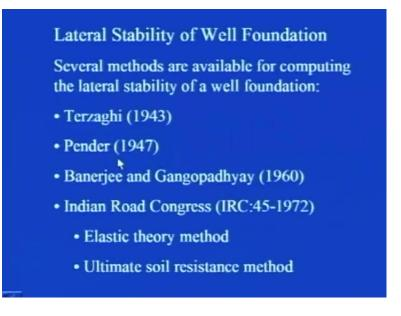
Now, coming to once we have the idea, about these forces and then how we can go for the stability analysis of this well foundation. Now, we have to see that, what all are the various methods which are available for the lateral stability of well foundation because, you know that it is a monolithic and a very rigid structure and its longer dimension is in the vertical direction and that is, why the lateral stability becomes quite important.
