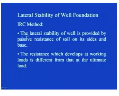
So, in IRC it says that, the lateral stability of well is provided by passive resistance of soil on its sides and base. The resistance which develops at working loads is different from that at the ultimate load that is, so obvious and it has been associated in recommendation by IRC also.
