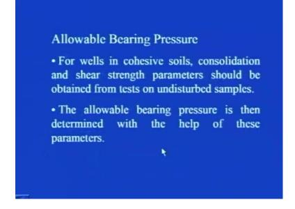
For wells in cohesive soils, consolidation and shear strength parameters should be obtained from the test on undisturbed samples. When you know that, where the foundation has to be laid, you can definitely collect the undisturbed sample and carry it to the laboratory and then conduct the test, to determine this shear strength parameters; that means, cohesion an angle of internal friction and then we use consolidation characteristic like coefficient of consolidation etcetera.
