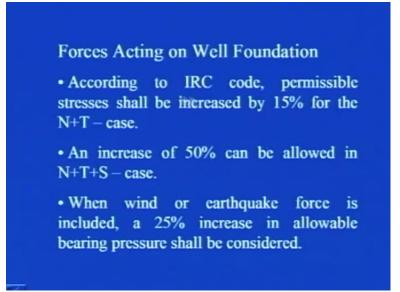
Now, according to IRC code, permissible stress shall be increased by 15 percent for the N plus T case then, an increase of 50 percent can be allowed in N plus T plus S case. When wind or earthquake force is included a 25 percent increase in allowable bearing pressure shall be considered. So, these are IRC recommendation which you have to follow.
