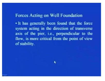
It has generally been found, that a force system acting in the direction of transverse axis of the pier, that is perpendicular to the flow is more critical from the point of view of stability because, two horizontal forces are there, that is P and Q, so which one to consider. So, usually it has been seen, that the force system which is acting in the direction of transverse axis of pier, that is opposite to the flow is more critical, so it is considered in the stability analysis.
