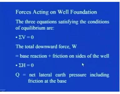
Then, for the stability analysis, you know from the mechanics point of view that, we usually require to satisfy equations of equilibrium. So, exactly the same thing we are going to do here in the case of well foundation also, so the three equations which satisfy the equation of equilibrium they are, first one is summation of all the forces in vertical direction is equal to 0.
