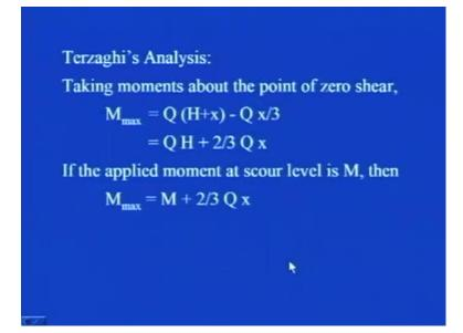
Then, taking moments about the point of zero shear because, that will be the point about which the maximum moment will be occurring and you know that, in the analysis and design procedure we always go for the maximum force and the maximum bending moment. So, M maximum you can obtain as Q H plus x minus Q x by 3, which will result into this particular expression as Q H plus 2 by 3 Q into x.
