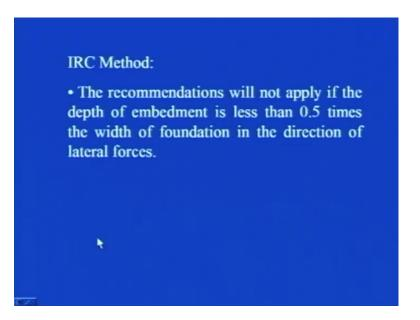
Then the recommendations will not apply, if the depth of embedment is less than .5 times the width of foundation in the direction of lateral forces. So, this is the limitation of this IRC method that, the depth of embedment if it is less than 0 point.5 times the width of the foundation in the direction of lateral forces then, these recommendations by IRC will not hold.
