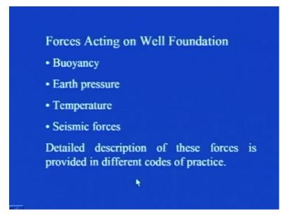
Further, due to the presence of water buoyancy force will be coming; further, earth pressure will be coming on the well foundation then, the force due to temperature and very well known seismic forces because, wherever it is earthquake prone area seismic forces will come into picture. Then detailed description of all these forces are available in the relevant IS codes or IRC recommendations.
