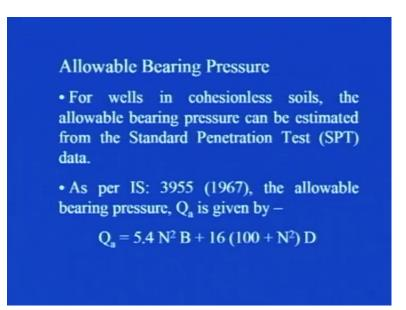
For wells in cohesionless soils, the allowable bearing pressure can be estimated from a standard penetration test data. As you have already studied in the very beginning of this particular course, what are the various field test and how the data of those field test can be used in the analysis and design of various foundations. So, the standard penetration
