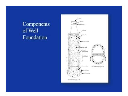
So, here is the different components of the well foundation, just you can have a look on this, that this top part that is the girder bearing pier cap and here is, this is the pier. These form, the super structure and the load from this, that is from the girder it comes to bearing, then the bearing transfers the load to pier cap and then it comes to pier. And just in contact with the pier, the first component of the well foundation comes, that is the well cap.
