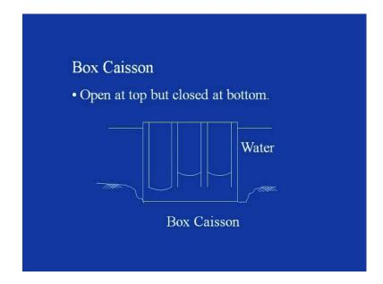
Here you can see the typical figure line diagram, explaining the box caisson features the top is open but the bottom is closed, these are some of the features of this type of caisson is that.
