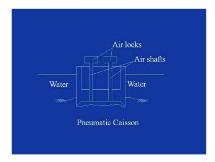
You can see here, that at the top two air locks are being provided, air shafts are being connected to this air lock and this goes inside the, it creates the pressure with the help of the air and that takes out the water and such that, here the dry condition is being carried out.
