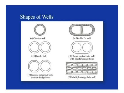
In this particular figure is the circular well, then the second one is double D-well, you can have dumb-bell shape, then fourth one is broad necked twin wells with circular dredge holes, double octagonal with circular dredge holes, then the last one is multiple dredge hole well. Now, let us see that the, what are the advantages and disadvantages of these different shape of well, in what condition these are preferred in what condition these are not employed.
