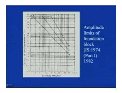
You can see here, that this is point A, this is D and prime, this figure has been taken from IS 1974 part 1 1982. So, this line, you can see here, that A D D prime, here on the X axis, you have disturbing frequency, on Y axis, it is amplitude of vibrations in micrometers. So, if you have ((Refer Time: 28:03)) that lower amplitude is required, that is for the, of disturbing frequency exceeding 20 hertz, then the value correspondingly, can be picked up from this particular line.
