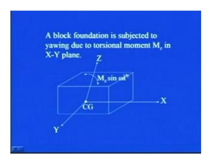
So, you can see here, that this has been shown, this block has been shown here and then, this is X axis, Y axis and Z axis and along Z axis, the rotation has been given, that is a moment has been given, that is of the magnitude of M z sin omega t. So, a block foundation is subjected to yawing, due to torsional moment M z in X Y plane, along Z axis.
