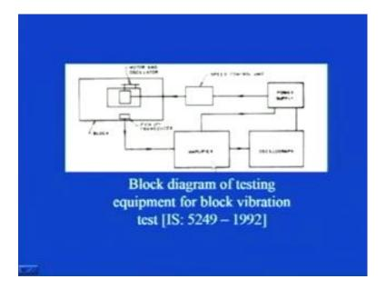
Then, this is the block diagram of testing equipment for, block vibration test, this is again has been taken from 5249, 1992, that is IS code, it is this concrete block. So, you can have a look that, how it looks from the top, so this is the concrete block, on top of that, this is the motor and oscillator, which has been mounted, here is the amplifier, here is the power supply, this is speed controller unit, so and here, it is transducer, to take the reading.
