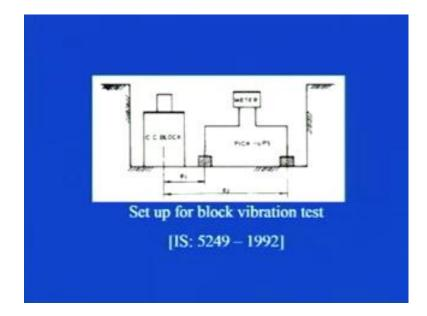
You can see here, that it, is the test pit, this is the figure, which has been taken from IS 5249, 1992. So, this IS code, if it is available to you, you can directly get, this particular figure from that, IS code, so this is, this shows the set up for, block vibration test, as I told you, that it is to be conducted in, a test pit. You see, this is the test pit, that is, at this particular depth from the ground surface you are planning to place the foundation for, that particular machine.
