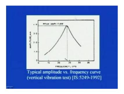
Now, you see here, that you have plotted, amplitude verses frequency curve, this is for one typical eccentricity value. So, that is why here, I am writing as, typical amplitude verses frequency curve, so for one particular eccentricity value, you can get, this amplitude for corresponding different frequency. So, what will happen, when the frequency is less, first it will go on increasing, and then it will attain, a peak value and after that, it will go on reducing.
