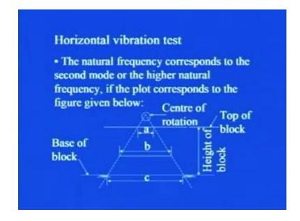
However, if the case is reverse that is like this, centre of rotation is here, this is height of the block, which we are plotting the variation, with this is top of the block, and you see that the variation is, in this manner. So, in this case, it is the, the natural frequency corresponds to the second mode or the higher natural frequency, if that particular plot corresponds to, this particular type of figure.
