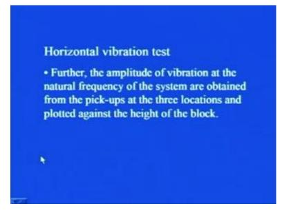
Exactly, on the similar lines, further, the amplitude of vibration, at the natural frequency of the system, are obtained from the pickups, at the three locations, and plotted against, height of the block So, the amplitude the vibration, at once, we you know the natural frequency, you can note down the amplitude of the vibration, then you have mounted, the pickups, acceleration pickups, at three locations, at it top, middle and the bottom, so that, you can plot, against the height of the block.
