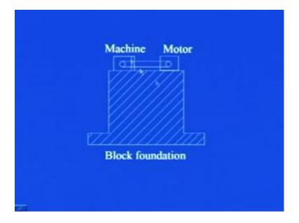
So, you see, you can see here, this is the pictorial view of block foundation, you see it forms kind of block, and on this one this machine as well as the motor, they are mounted, it is mass is quiet high, and so it is natural frequency is less.
