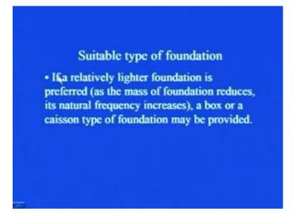
Now, if the relatively lighter foundation is preferred, because when the mass of the foundation reduces, it natural frequency increases. So, in case, you require such type of foundation, that you want more natural frequency, so in that case, you have to reduce the mass of the foundation. So, in that case, a box or a caisson type of foundation may be provided.
