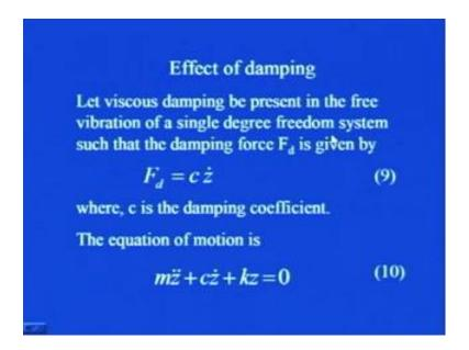
Now, I assume that, the viscous damping is present in the system, so first we talk of, free vibration of single degree freedom system, as we did, in earlier case, when the damping was absent we, analyze for free vibration and then we went for, the forced vibration. So, likewise in, when we are studying, this effect of damping then also, we first considered, that it is free vibration of a single degree freedom system, such that, the damping force F d, d this subscript, d stands for this damping.
