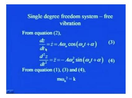
So, from the previous equation, you can get that, differentiating it once, that the d z d t is z dot, is equal A w n sorry, omega n cos omega n t plus alpha. Then, if you further
