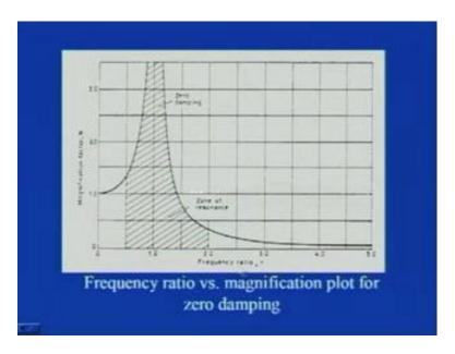
That on x axis, it is the frequency ratio, on y axis, it is magnification factor, so incase, the frequency ratio becomes 1. So, you see, if r is becoming 1, then 1 minus r is square will become 0, and the n, which is defined as 1 upon, 1 minus r square will tend to infinity. So, you can see here, that incase, when the r is equal to 1, the curves they are becoming, ((Refer Time: 37:35)) here, in this particular region, and they are tending towards infinity.
