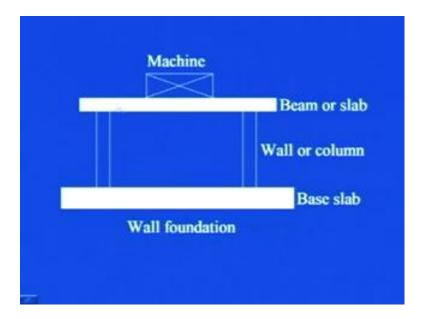
You see here, this is beam or a slab, this is wall or column, and this is base slab, which will be resting on the soil. So, that comprise of, you can see here, that each and every, part of this particular system, they are, although they are integrated together, to form this wall foundation. But, if you have a look, on the individual columns they are quiet, on the individual component of this particular foundation, they are quiet flexible, and on top of that this machine is mounted.
