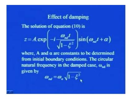
Then, it is solution, although you can derive this solution, but that is beyond the scope of your, this particular course. So, its equation, you can simply get that as, z is equal to A into exponential minus i omega n d, n d stands for natural frequency of the damped system, into t divided by square root of 1 minus zeta square, sin omega n d t plus alpha. Now, this A and alpha they are constants, to be determined from initial boundary conditions.
