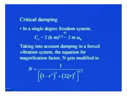
Then, how you can define it, that in a single degree freedom system, the critical damping is defined as, twice square root of k into m, and you know, that omega n square was equal to that k by m. So, you substitute it here, so you will be simply getting, here that omega n square, if you substitute here, so you will be getting, the 2 into m into omega n, taking into account, damping in a first vibration system, see right now, we were talking, in terms of free vibration now.
