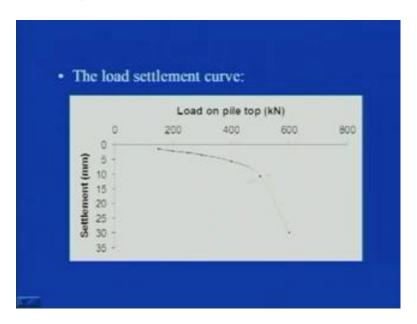
So, this is load on pile top in kilo Newton settlement it has been plotted, which follows this particular curve. So, it has been asked in the question that you have to plot this load settlement curve, so this is how you can plot the load settlement curve, first you find out the elastic settlement and then correspondingly simply using may be graph sheet or this I have done in excel, there you can plot this load settlement curve.
