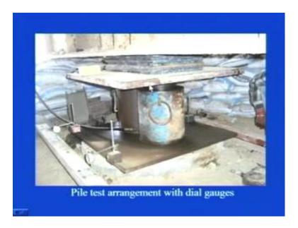
So, you can see here earlier you saw the arrangement which has to be done for conducting this initial test, above the ground surface. Now, how that particular load is being transferred to the pile that you can see here in this particular picture, that this is what is the pile cap that is above the existing ground surface over here, in the pit and then minimum of three dial gauges are to be provided to measure the settlement corresponding to any particular load.
