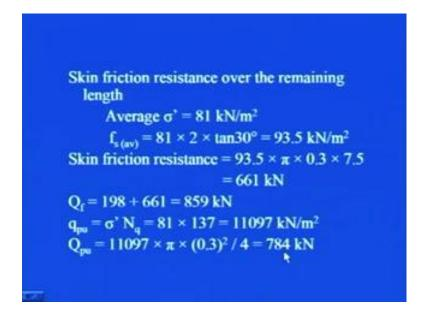
Then, skin friction resistance over the remaining length, so beyond 4.5 meter till the length of the pile, this average sigma prime will be constant which is equal to 81 kilo Newton per meter square. And so this f s average will become 81 into K that is 2 into tan delta, delta is 30 degree and this will result into 93.5 kilo Newton per meter square.
