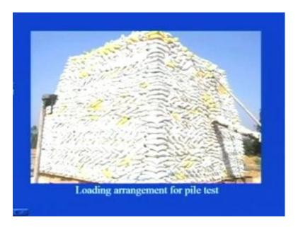
You see this is another view of that loading arrangement because, you know at a time you have to mobilize lot of I mean quite heavy amount of load, depending on the type of the structure, this is what is in the test conducted at a site, where the cement plant was coming up. So, in case of cement plant all the heavy structures they come up, so load coming on the pile they are quite high, so you have to mobilize that much high load, so for that you have to have that much of the bags.
