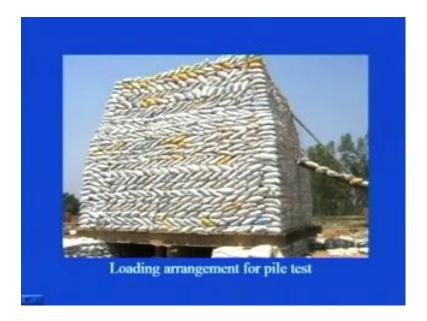
So, you see here this is what is the loading arrangement for pile test, you can see here that the girders are placed in this at regular interval to frame a loading platform. And on which these bags filled with soils they are placed, you know that in usual language they labors they call it as ((Refer Time: 30:48)) So, all these bags, they are filled up with soil and the weight of each bag is approximately 30 kg's or so.
