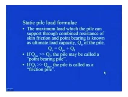
Then, the maximum load which the pile can support through combined resistance of skin friction and point bearing is known as ultimate load capacity, which we represent usually by Q u of the pile. So, whatever is the distribution or how it is getting transferred, whatever the load which is coming on the pile; that is compressive load from super structure.
