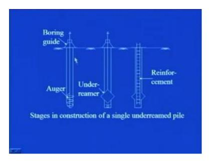
So, you see here with the help of figure, if I explain you, so first this hole is prepared that is called bore hole, that is boring guide with the help of this, you insert it the auger, see it is of this kind of shape. Now, what happens is with the auger, you just put the rotary action and then you take out the soil. So, this is the process of preparing this bore hole, once this bore hole is prepared, you insert the under reamer.
