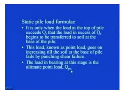
That the load in excess of Q f, begins to be transferred to soil at the base of the pile, so you see the load is gradually increasing and from there a situation will come, when this friction load will get mobilised, along the total length of the pile shaft. And that particular stage, we are calling as ultimate skin friction resistance Q f, so at that particular situation or condition, your Q which is applied from the top will become equal to Q f.
