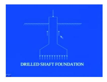
Another example in this cases the drilled shaft foundations form it is use may be bridge pear and for other structures.
