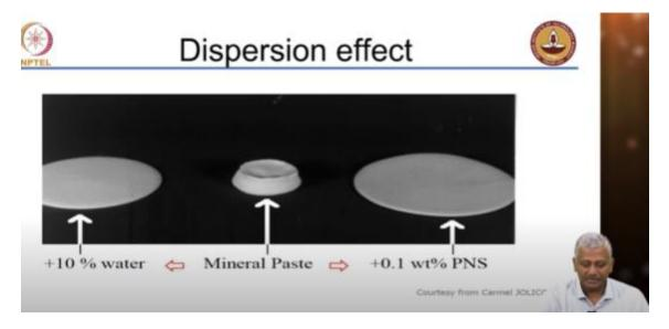
Now just to revisit the effect of dispersion in a very simple way, if this is a cement paste that is formed with just water and cement, if you add extra water you make it more flowable but you do not add extra water you just add the super plasticizer in this case poly naphthalene sulphonate only about 0.1% can make it more flowable than adding extra water.
