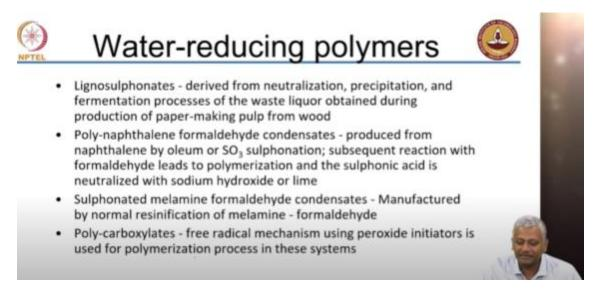
Lignosulphonates as I said, you are getting the lignite from the wood. It is basically the waste liquor that is obtained during the paper manufacturing process. Paper is basically you extract the cellulose out of the wood so lignin remains and you are leading to neutralization, precipitation, fermentation processes that lead to the ultimate production of lignosulphonate based chemicals.
