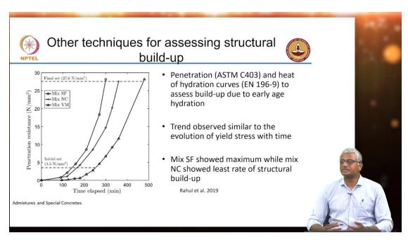
And you can also instead of using a vane shear to determine yield stress and measure the build-up with respect to yield stress, you can also substitute that with a simpler technique like penetration, which we use for setting time determination, penetration resistance test could also be used for determination of how 3D printed materials are building up an internal stress.
