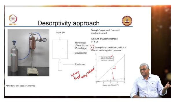
So, we adopted this test methodology which is typically used for water retentivity of mortars.
