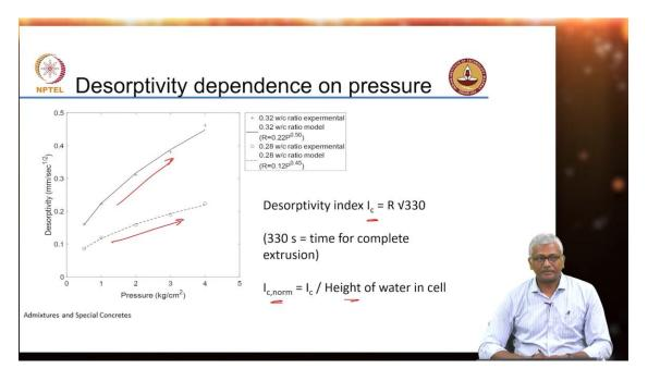
So, here the desorptivity coefficient is obviously dependent on the pressure. As the pressure increases the coefficient also increases. So, based on this value we actually came out with what is known as a desorptivity index which again was taken as R times square root of 330 where 330 seconds was the time for complete extrusion of the mix. And then we normalized the entire value that is obtained here by dividing by the height of water in the cell.
