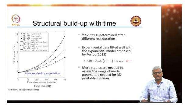
And for all these mixtures the structural build-up, and internal build-up we discussed earlier how this internal build-up is important because the internal yield stress has to build up to a level that is able to overcome the stress due to the weight of the additional layers that come on top. So, we have to understand this behavior also, and as I was telling you earlier there are non-linear rheological models which can help you fit this equation also.
