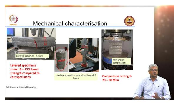
Now the difficulty comes in the mechanical characterization of 3D printed materials because it is no longer going to be possible for you to characterize the strength just based on a cube or a cylinder.
