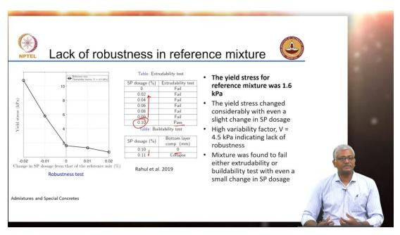
So, in this reference mixture, there was an absolute lack of robustness. So, if the dosage was exactly 0.1% it was passing the extrudability test and it was passing the buildability test also. There was no deformation in the bottom layer. But going less than 0.1 made the mix fail the extrudability test which means the filament that came out did not have a very
