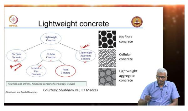
In general, lightweight concrete can be classified into no fines concrete. Why is no fines concrete lightweight? Because we are not adding any sand. So obviously there will be a lot of void spaces present in the system. No fines concrete is also christened as pervious concrete in certain literature.
