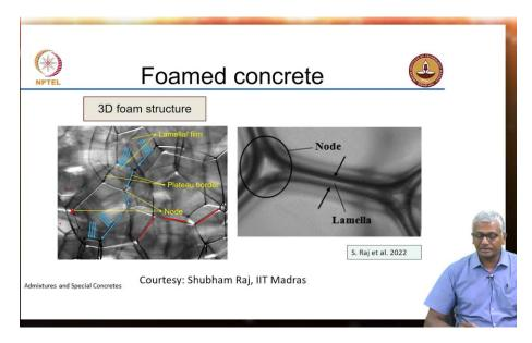
This shows you the foam structure, the structure of the foam itself under a microscope. So, you can see very clearly each individual bubble and the joining bubble next to it.
