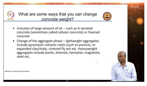
Now how do you make concrete change weight? The maximum proportion of material inside the concrete belongs to aggregate. So, by making aggregates lightweight or heavy weight is the easiest way that you can change the density of the concrete. Alternatively, if you want to make concrete lightweight you can also introduce more air in the system.
