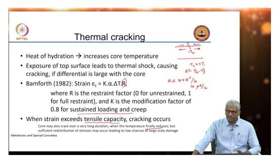
This is primarily from the perspective of thermal cracking and the thermal cracking can be of two types, one that arises because of temperature differentials between the core and the surface, the other which happens because you have internal problems such as delayed trigger formation that may happen at very high temperatures.
