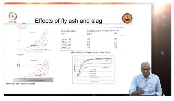
Now again needless to say when you use fly ash or slag you get extremely beneficial conditions for mass concrete. Now we also saw earlier that there is cements like low-heat cements that are potentially available which has higher C2S and low C3S content but for a cement company to produce low-heat cement requires a major change of their process and many cement companies are not ready to do this. For them, it is much easier to do this
