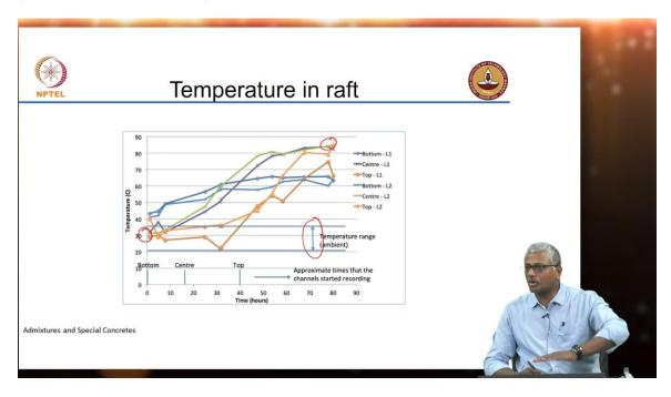
This is again more consolidated temperature in the raft. As I said the temperature in the core had reached up to about 85 to 90 degrees Celsius, a significant temperature rise. But you can see here that the placement temperatures as per the spec the placement temperatures were allowed up to 30 degrees Celsius.
