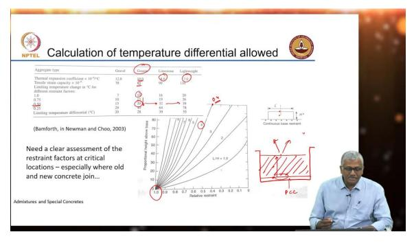
Now as we see from the table, I showed you previously in some instances depending on the extent of restraint even a lesser amount of temperature difference can result in cracking.
