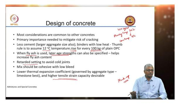
So, again most considerations for the design of raft concrete are similar to other concrete. But then all these aspects about temperature differentials, generation of high temperature in the core, all these have to be looked at carefully. So minimizing or mitigating the risk of cracking is absolutely important.
