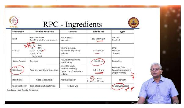
So, ingredients typically sand as I said less than 600 micron, cement we want to choose cements that are high in  $C_3S$ . Of course, this is not necessarily true  $C_3S$  of 3.8% happens only in sulphate-resistant cement which we typically would not get such low  $C_3S$  in normal cement.
