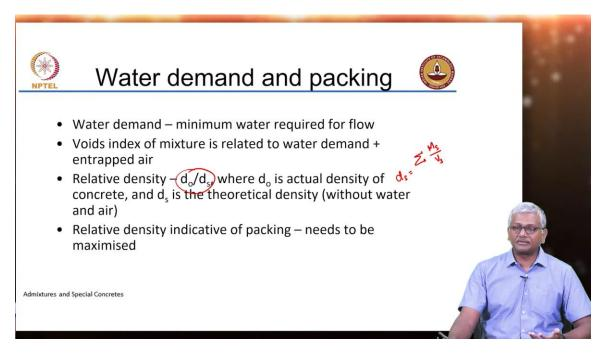
So, as I said again you are employing concepts of particle packing where you can define a parameter such as relative density  $d_0$  by  $d_s$  where  $d_0$  is the actual density of the concrete which is achieved after compaction and  $d_s$  is the theoretical density without the consideration of any voids.
