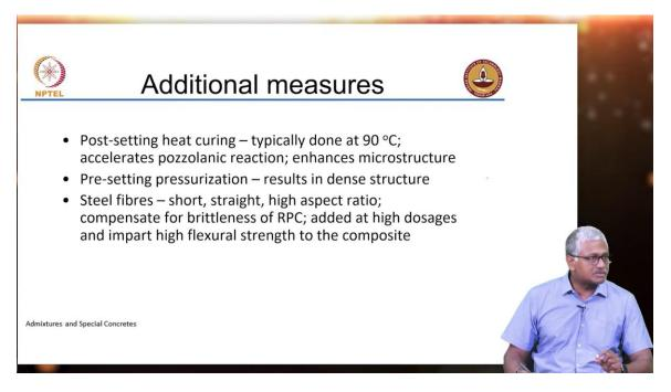
Post static heat curing typically done at 90 degrees Celsius. It is a very high temperature, 90 degrees is a very high temperature, it cannot be sustained for a long period of time.
