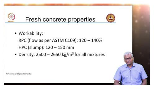
The range of workability that was desired was in terms of flow in reactive product concrete and slump in high-strength concrete or high-performance concrete.
