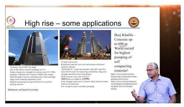
Some examples are given here. This tallest concrete building in the US about 70 stories 82.7 MPa. This is one of these buildings. I think it is the South Packard Drive building in Chicago and again about 84,000 cubic meters of concrete was poured here.
