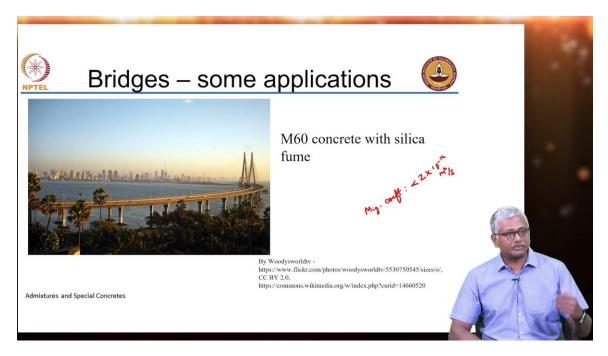
Of course, one popular structure in India is the Bandra-Worli sea link. Again here M60 concrete with silica fume is used for the piers that you see. The piers of the bridge were made with M60 concrete with silica fume.
