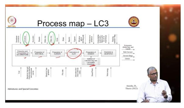
In LC3 you have instead of fly ash being one ingredient now you have two other ingredients, one extra limestone and extra calcium clay. So, here extra processes are involved, again limestone extraction and transportation fine. Then you have preparation of raw meal, then you have preparation of clinker, then you also have to include the calcination of clay.
