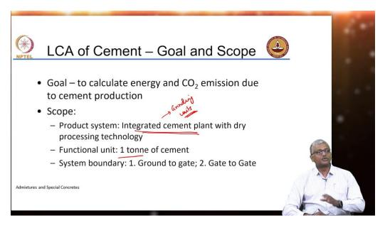
Now in this case for the example that I have chosen here we are trying to do a life cycle assessment of cement. The goal is to calculate energy and  $CO_2$  emission due to cement production. So, it is defined in such simple terms just to calculate the  $CO_2$  and energy emission due to cement production. The scope, the product system is an integrated cement plant which has a dry processing technology. What is a dry process plant? In the old days, people were using wet process plants.
